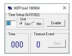
The demo software, you can set the Watchdog timer times, example you use default 10 seconds watchdog timer, when you press "Enable" button, after 10 seconds final count down, it will execute watchdog reset signal.
