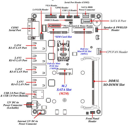
\*Note: SIM card slot only work when compatible SIM card installed & 3G LAN card installed in MPE2 Mini-PCIE slot.
