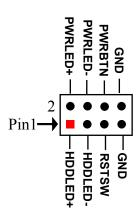
(2) SPK-LED1 (8-pin): Speaker & Power LED Header
