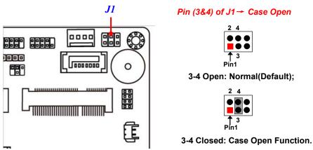
**Pin (3&4) Closed**: When Case open function pin short to GND, the Case open function was detected. When used, needs to enter BIOS and enable 'Case Open Detect' function. In this case if your case is removed, next time when you restart your computer, a message will be displayed on screen to inform you of this.
