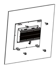
4. Mount the Panel PC system into the pre-cut space of the wall plane, as the photo shows.
