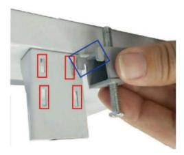
Insert corresponding edges of the fixed part into the slots of metal support until them matched. Make sure the fix part is installed in the way the photo shows, with protruding tips upwards. User can choose the height of installing spot.
