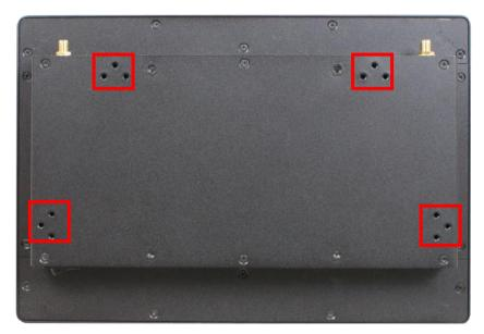
1. **Back side:** Find the marked spots with 3 reserved screw holes are for installing the optional fixed parts.
