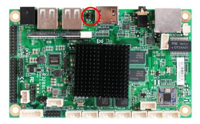
\*Note: OTG\_JP is in the marked position. User can select OTG or USB 2.0 function by jumper setting.
