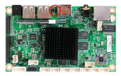
\*Note: OTG\_JP is in the marked position. User can select OTG or USB 2.0 function by jumper setting.
