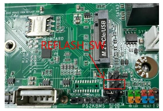
6. REFLASH\_LED light will turn green, which indicates system is checking BIOS files in the USB disk for updating. When re-flashing the BIOS, LED light will keep flashing on. The whole BIOS re-flashing process will takes about 6 minutes.
