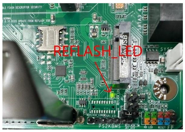
7. When BIOS re-flashing completes, the system will restart automatically and LED light will turn off, which means BIOS update is complete.
