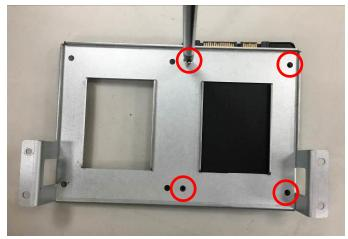
4. Turn over the tray and lock the 2.5"HDD to the tray by tightening up the marked screws as the photo shows.
