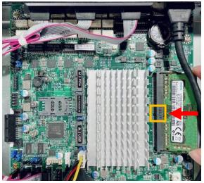
2. Insert the gold-finger side of the compatible SO-DIMM into the slot at a 30 degree angle. See to it that the break of the module fit into the notch of the slot.
