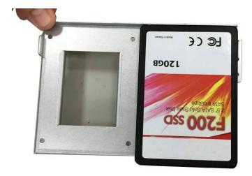
3. User can install up to 2\*2.5" HDD on the tray. Adjust the 2.5" HDD on the tray until the screw holes of the tray matched those in the HDD. (Support 2.5" HDD with a height  $\leq 10$ mm)
