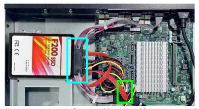
6. Connect one end of compatible SATA cable to corresponding connectors from the hard disk, and connect SATA Power cable and the other end of SATA cable to SATA port on the board as shown above.
