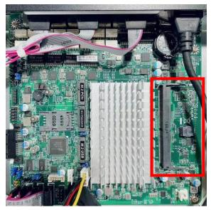
1. Locate the SO-DIMM memory slot on the board.
