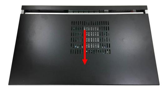
3. Push the top cover of the chassis towards the direction as the photo shows. Then lift the cover up to open the chassis.
