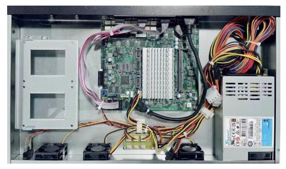
4. The overview of internal layout of the system for quick installation guide.
