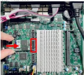
3. Insert the gold-finger side of the compatible M.2 M-key (2242) card into the slot at a 30 degree angle and press down.
