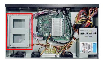
1. Locate the HDD tray on the chassis.
