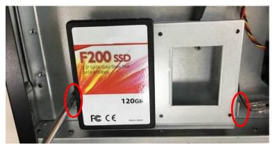
5. Put the tray with hard disk drivers installed to its original place and lock the tray to the chassis by tightening screws removed previously.
