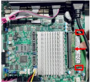
3. Press down to lock the SO-DIMM. The eject tabs will lock automatically if installing direction is correct.
