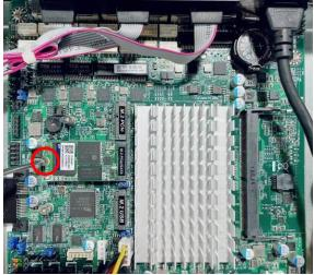
4. Lock the card to the board by tightening up the screw to the marked spot.
