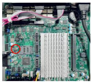
2. Remove the marked screw and use it to lock M.2 M-key (2242) card to the slot in later installation.
