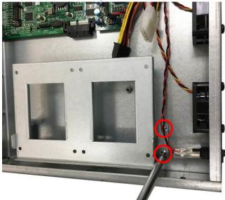
2. Remove the above marked screws that lock the tray to the chassis and pick them out of the chassis (4 screws in total on both sides).
