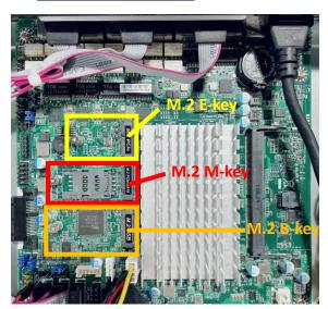
1. Locate the M.2 M-key SATA slot, M.2 E-key PCIe slot and M.2 B-key USB slot on the board.
