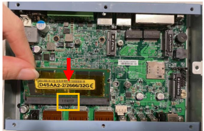
2. Insert the gold-finger side of the compatible SO-DIMM into the slot at a 30 degree.
