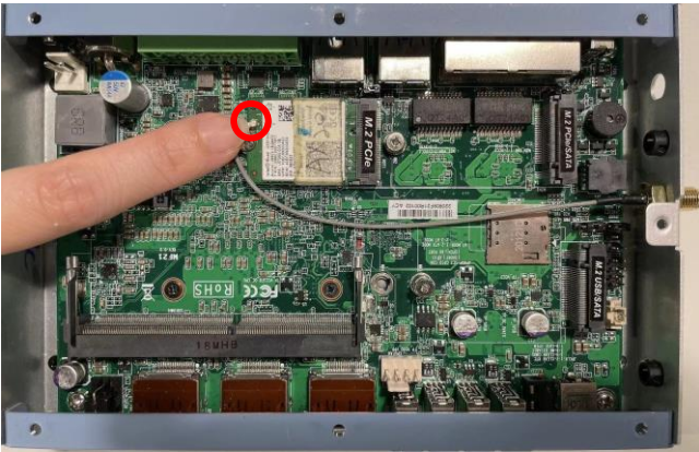
8. Press the metal hat on the end of the antenna string to corresponding antenna slot on the card as showed.
