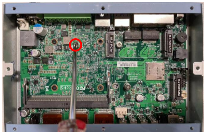
2. Remove the marked both screw and screw bolt, and use screw bolt to lock compatible card to the slot in later installation.
