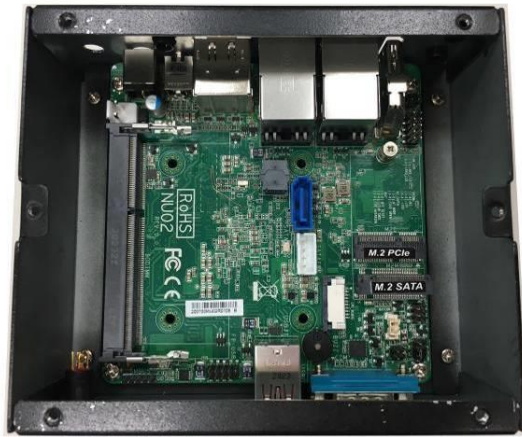
2. The internal structural view of the system for further intallation.
