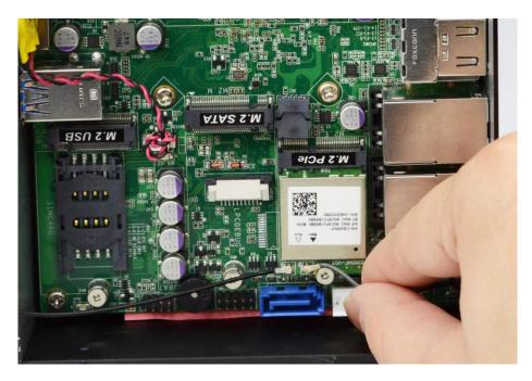
8. Press the metal hat on the end of the antenna string to corresponding antenna slot on the card as shown.
