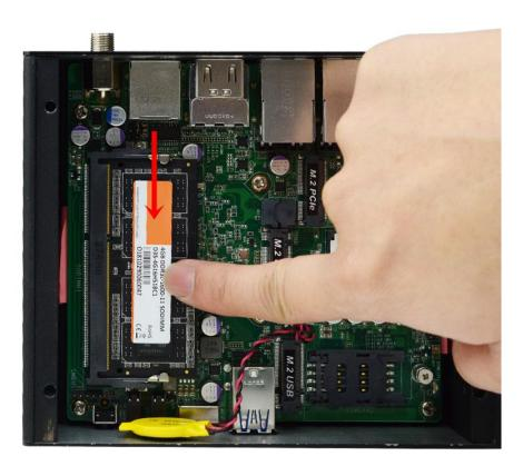
3. Press down to secure the SO-DIMM to the slot. The eject tabs will lock automatically if installing direction is correct.
