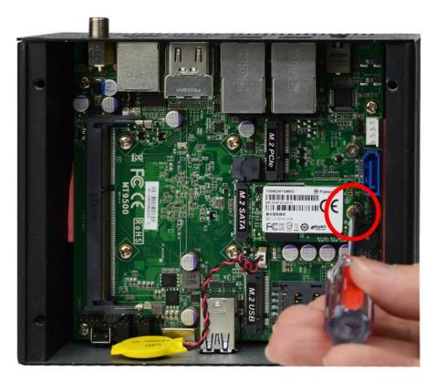
4. Tighten up the screw removed before to the marked spot to secure the card.
