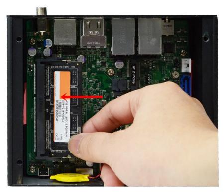
2. Insert the gold-figure side of the compatible SO-DIMM into the slot at a 30 degree.
