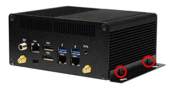
1. Install wall mount rack to the system by tightening two screws in the marked positions.
