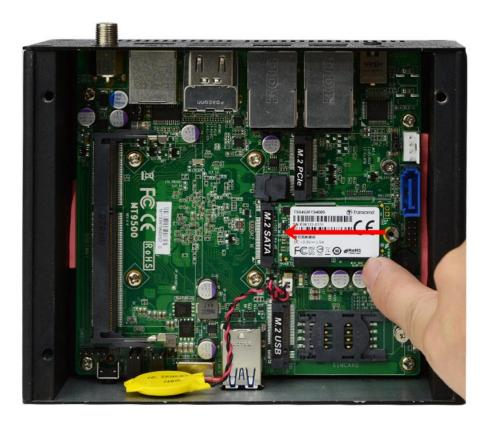
3. Insert compatible 2242 card into the slot.
