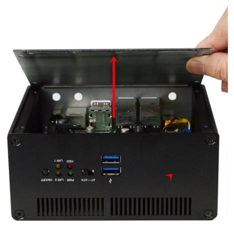
2. Lift the cover up to open the chassis.
