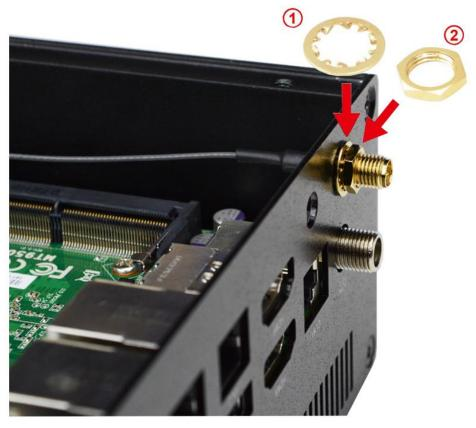
7. And then lock the antenna head to the front side of the rear panel with the hexagonal screwnut ② and tighten it up.
