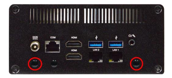
5. Locate the reserved antenna holes on the back panel. Remove the dust-proof plugs on the marked spots from the panel to install the antenna, as the following details show.
