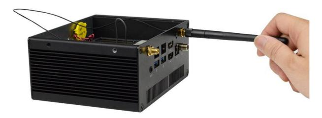
10. Connect the external Wi-Fi receiver antenna to the antenna screw head on the rear panel.
