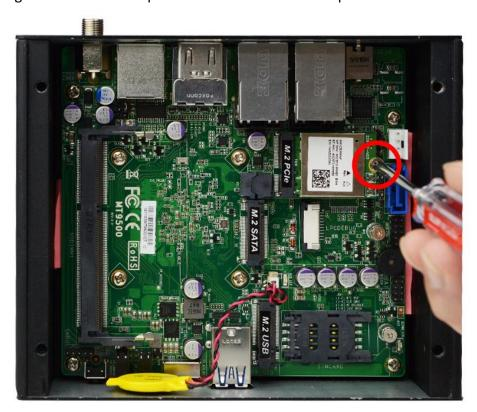
4. Secure the card to the board by tightening up the screw to the marked spot.
