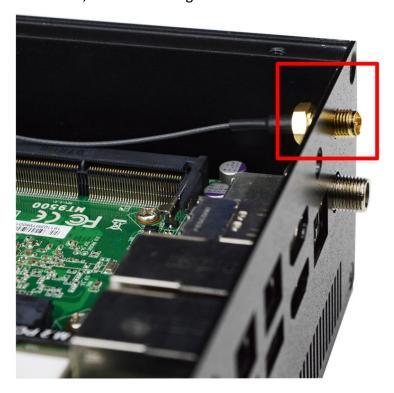
6. Push this antenna head into antenna hole of the rear panel from the backside of the panel.
