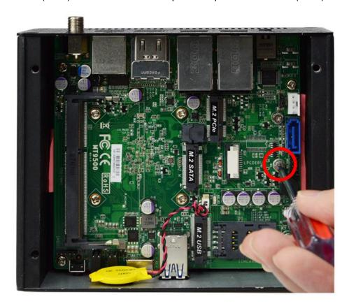
2. To install compatible card, please remove the screw in the marked spot at first.
