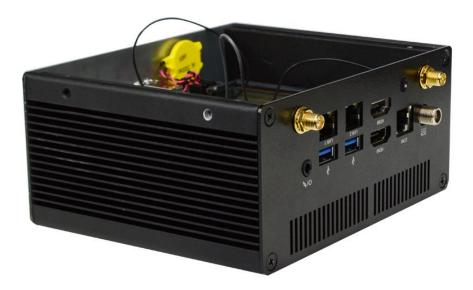
9. The rear panel with antenna screwheads installed.
