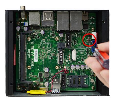
2. Remove the marked screw and use it to lock compatible card to the slot in later installation.
