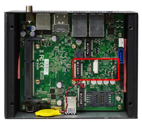
1. Locate the M.2 SATA (2242) slot on the board. Prepare compatible M.2 SATA (2242) card.
