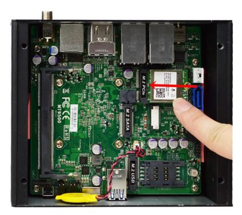
3. Insert the gold-figure side of the compatible card into the slot and press down.
