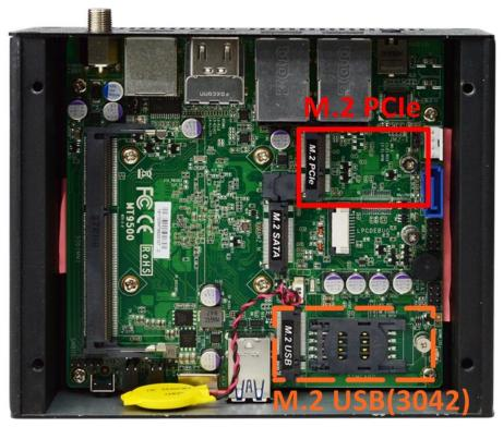
1. Locate M.2 PCIe slot on the board.
