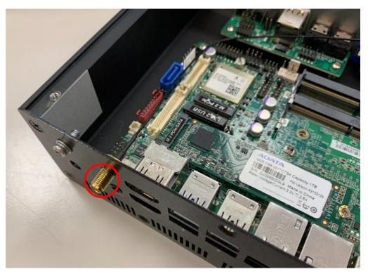
6. Push this antenna screw head into antenna hole of the rear panel from the backside of the panel.
