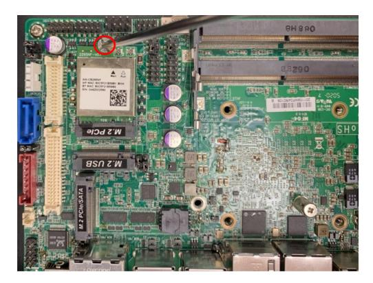
4. Secure the card to the board by tightening up the screw to the marked spot.
