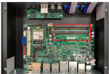
1. Locate the SO-DIMM slot on the board.
