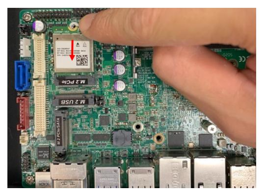
3. Insert the gold-figure side of the compatible card into the slot and press down. See to it that the golden-finger side should be fully plugged into the slot.
