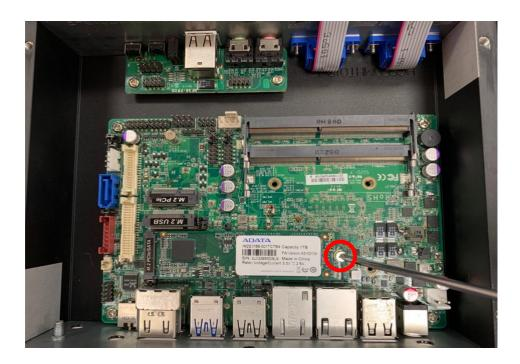
4. Secure the card to the board by tightening up the screw to the marked spot.
