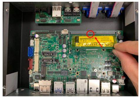
2. Insert the gold-figure side of the compatible SO-DIMM into the slot at a 30 degree angle. See to it that the break of the module fit into the notch of the slot and the golden-finger side should be fully plugged into the slot.
