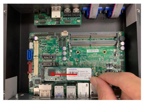
3. Insert compatible M.2 PCle (2280) card into the slot. See to it that the golden-finger side should be fully plugged into the slot.
