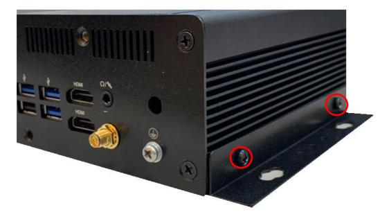
1. Install wall mount rack to the system by tightening two screws in the marked positions.
