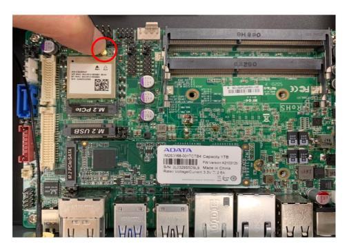
8. Press the metal hat on the end of the antenna string to corresponding antenna slot on the card as showed.
