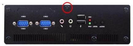
2. Remove the marked screw on the front IO panel.
