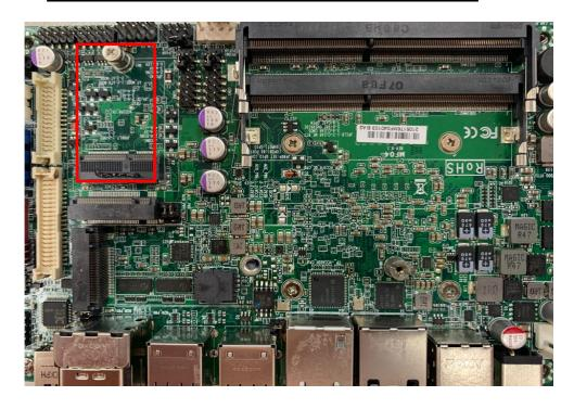
1. Locate the M.2 E-Key PCle (2230) slot on the board. Prepare compatible M.2 E-Key PCle (2230) card.
