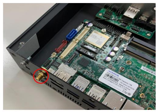
7. And then lock the antenna screw head to the front side of the rear panel with the hexagonal screw nut ② and tighten it up.
