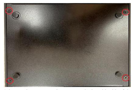
1. Locate the screws at the spots marked on this side of the system and unscrew them one by one.
