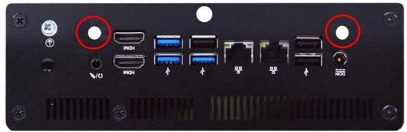
5. Locate the reserved antenna holes on the rear panel. Remove the dust-proof plugs on the marked spots from the panel to install the antenna.
