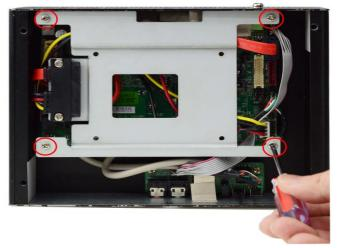
6. Remove the marked screws to dissemble the HDD tray from the system.
