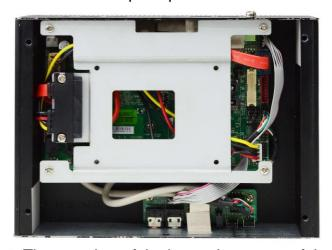
5. The overview of the internal structure of the system with HDD tray pre-installed.
