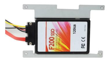
1. Place compatible SATA HDD upon HDD tray as showed above. Plug this side of the cable to SATA power-in connector and SATA connector of the hard disk.
