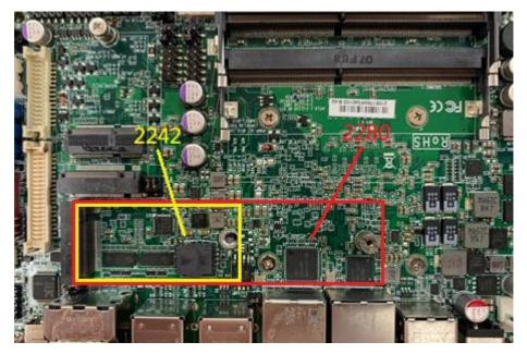
1. Locate the M.2 M-Key SATA (2242/2280) slot on the board. Prepare compatible M.2 M- Key SATA (2242/2280) card.
