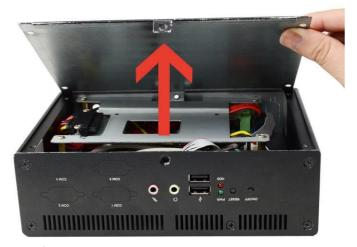
4. Lift the cover up to open the chassis.
