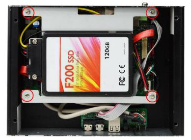
4. Adjust the installed tray as showed above. Fix HDD tray into the system by tightening up 4 screws marked. (refer to I-6)
