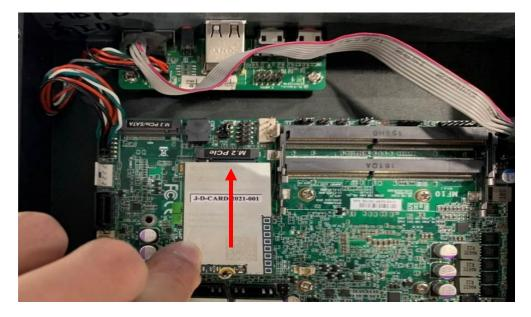
3. Insert the gold-figure side of compatible M.2 B-Key, type-3052 card into the slot until the golden finger side fully emerged into the slot.
