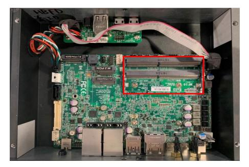
1. Locate the SO-DIMM slots on the board.
