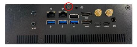
3. Remove the marked screw on the rear IO panel.
