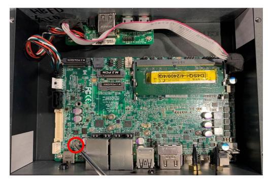
2. To install compatible card, please remove the screw in the marked spot at first.
