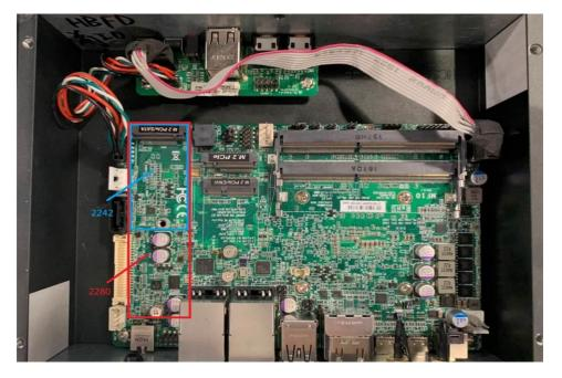
1. Locate the M.2 SATA slot on the board. System supports two types of M.2 M-Key card in different lengths (2280/2242). Prepare compatible M.2 SATA card.
