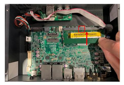
2. Insert the gold-figure side of the compatible SO-DIMM into the slot at a 30 degree angle. See to it that the break of the module fit into the notch of the slot and the golden-finger side should be fully plugged into the slot.
