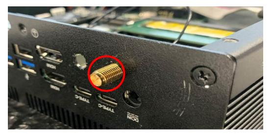
6. Push this antenna screw head into antenna hole of the rear panel from the backside of the 11
