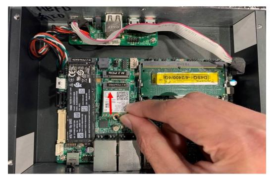
3. Insert the gold-figure side of the compatible card into the slot and press down. See to it that the golden-finger side should be fully plugged into the slot.
