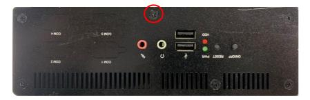
2. Remove the marked screw on the front IO panel.
