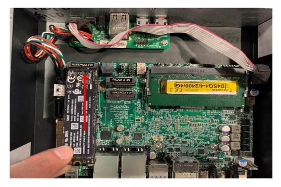
3. Insert compatible M.2 M-Key, type-2280 card into the slot. See to it that the golden-finger side should be fully plugged into the slot.
