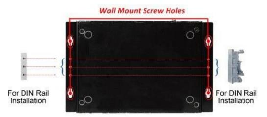
3. Wall mount the system by tightening 4 screws in the marked positions on both sides of the wall racks.
