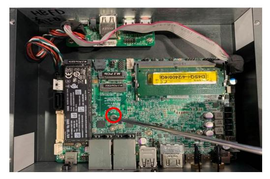
2. Remove the marked screw and use it to lock compatible card to the slot in later installation.
