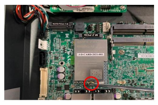
4. Install the screw back to the original spot.
