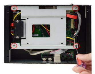
6. Remove the marked screws to dissemble the HDD tray from the system.
