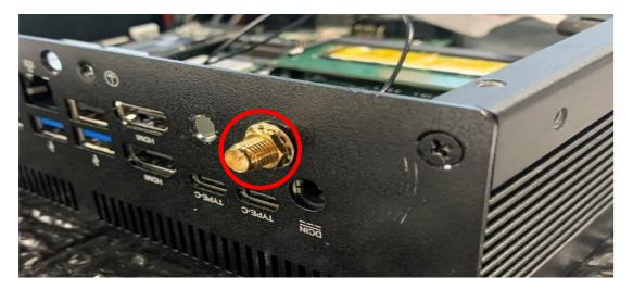
7. And then lock the antenna screw head to the front side of the rear panel with the hexagonal screw nut(2) and tighten it up.
