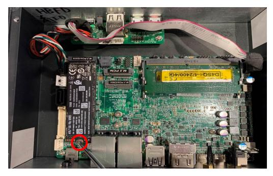
4. Tighten up the screw removed before to the marked spot to secure the card.
