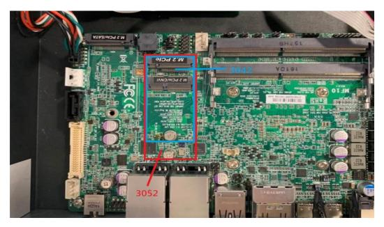
1. Locate the M.2 B-Key, type-3042/3052 slot on the board.
