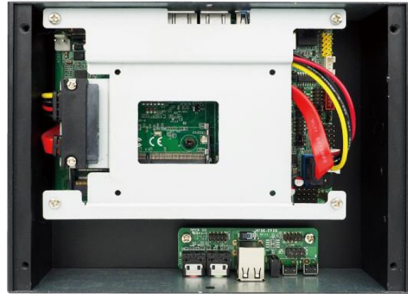
5. The overview of the internal structure of the system with HDD tray pre-installed.
