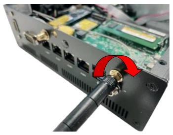
11. Connect the external Wi-Fi receiver antenna to the antenna screw head on the rear panel.
