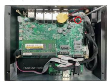
2. To install compatible card, please remove the screw in the marked spot at first.
