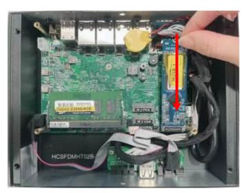
3. Insert compatible M.2 M-Key, type-2280 card into the slot. See to it that the golden-finger side should be fully plugged into the slot.
