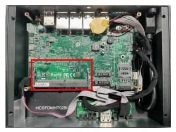
1. Locate the SO-DIMM slot on the board.
