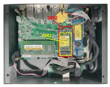
1. Locate the M.2 B-Key PCIe (3042/3052) slot on the board. Prepare compatible M.2 B-Key (3042/3052) card.
