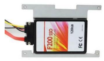
1. Place compatible SATA HDD upon HDD tray as showed above. Plug this side of the cable to SATA power-in connector and SATA connector of the hard disk.
