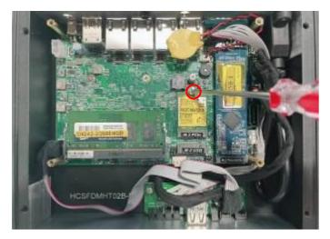
4. Secure the card to the board by tightening up the screw to the marked spot.
