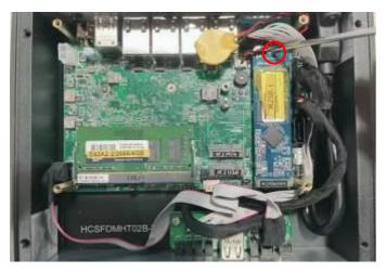
4. Tighten up the screw removed before to the marked spot to secure the card.
