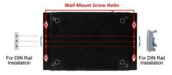
3. Wall mount the system by tightening 4 screws in the marked positions on both sides of the wall racks.
