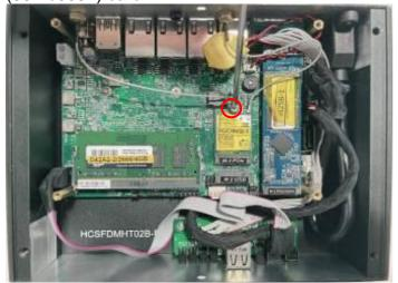
2. Remove the marked screw and use it to lock compatible card to the slot in later installation.
