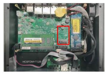
1. Locate the M.2 E-Key PCle (2230) slot on the board. Prepare compatible M.2 PCle, type - 2230 card.
