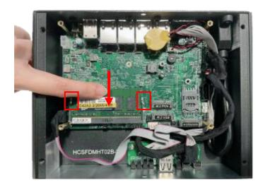
3. Press down to secure the SO-DIMM to the slot. The eject tabs will lock automatically if installing direction is correct.
