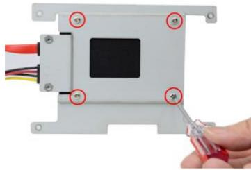
2. Turn over the HDD tray and fix 2.5" HDD upon HDD tray by tightening 4\* screws marked in corresponding spots.
