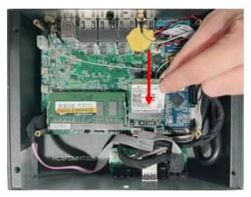
3. Insert the gold-finger side of compatible M.2 B-Key, type-3042 card into the slot until the golden finger side fully emerged into the slot.
