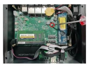
2. Remove the marked screw and use it to lock compatible card to the slot in later installation.
