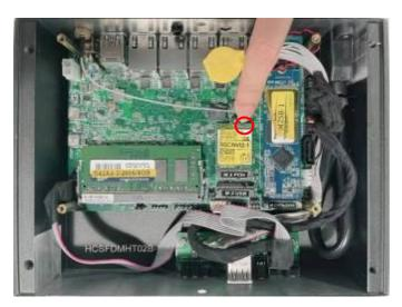
8. Press the metal hat on the end of the antenna string to corresponding antenna slot on the card as showed.
