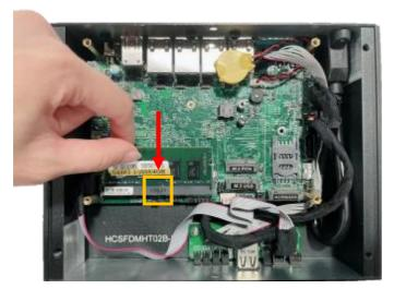
2. Insert the gold-finger side of the compatible SO-DIMM into the slot at a 30 degree angle. See to it that the break of the module fit into the notch of the slot and the golden-finger side should be fully plugged into the slot.
