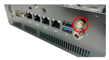
6. Push this antenna screw head into antenna hole of the rear panel from the backside of the
