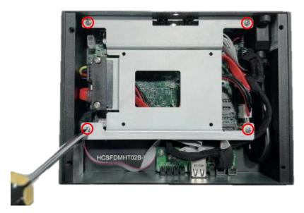
6. Remove the marked screws to dissemble the HDD tray from the system.
