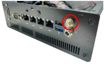
7. And then lock the antenna screw head to the front side of the rear panel with the hexagonal screw nut② and tighten it up.
