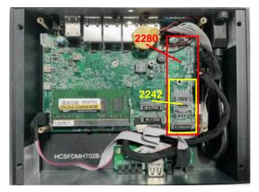
1. Locate the M.2 SATA slot on the board. System supports two types of M.2 M-Key card in different lengths (2242/2280). Prepare compatible M.2 SATA card.
