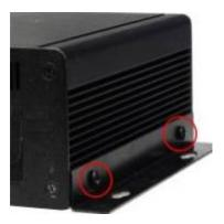
1. Install wall mount rack to the system by tightening two screws in the marked positions.
