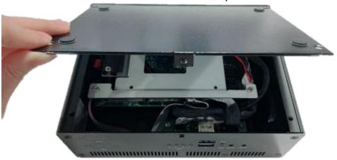
4. Lift the cover up to open the chassis.
