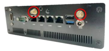
10. The rear panel with antenna screwheads installed.
