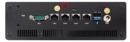
3. Remove the marked screw on the rear IO panel.
