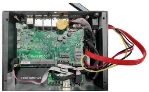
3. Plug SATA power connector and SATA port connector into connectors onboard.
