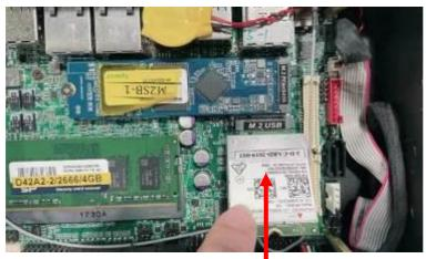
3. Insert the gold-finger side of compatible M.2 B-Key, type-3042 card into the slot until the golden finger side fully emerged into the slot.
