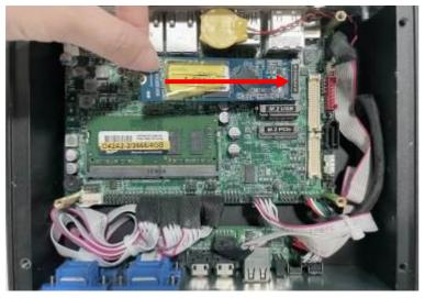
3. Insert compatible M.2 M-Key, type-2280 card into the slot. See to it that the golden-finger side should be fully plugged into the slot.
