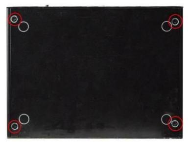
1. Locate the screws at the spots marked on this side of the system and unscrew them one by one.
