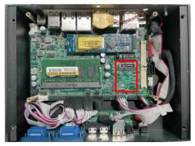
1. Locate the M.2 E-Key PCle (2230) slot on the board. Prepare compatible M.2 PCle, type - 2230 card.
