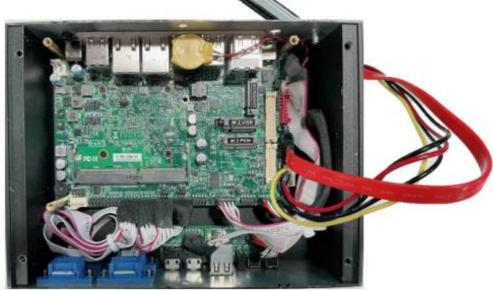
3. Plug SATA power connector and SATA port connector into connectors onboard.
