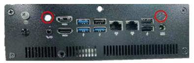
5. Locate the reserved antenna holes on the rear panel. Remove the dust-proof plugs on the marked spots from the panel to install the antenna.
