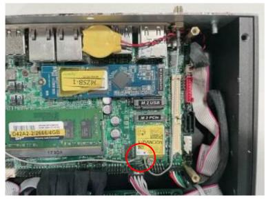
9. Repeat step 6 to 8, to finish installation of the other antenna.
