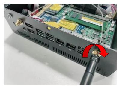
11. Connect the external Wi-Fi receiver antenna to the antenna screw head on the rear panel.
