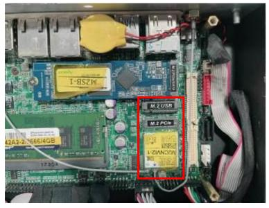
1. Locate the M.2 B-Key, type-3042 slot on the board.
