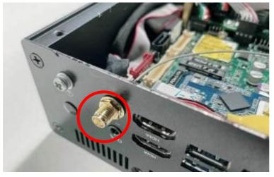
7. And then lock the antenna screw head to the front side of the rear panel with the
