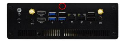
3. Remove the marked screw on the rear IO panel.
