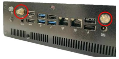
10. The rear panel with antenna screwheads installed.
