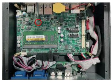
2. To install compatible card, please remove the screw in the marked spot at first.
