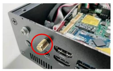
6. Push this antenna screw head into antenna hole of the rear panel from the backside of the panel.
