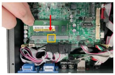
2. Insert the gold-finger side of the compatible SO-DIMM into the slot at a 30 degree angle. See to it that the break of the module fit into the notch of the slot and the golden-finger side should be fully plugged into the slot.
