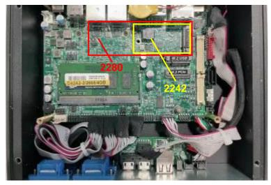
1. Locate the M.2 SATA slot on the board. System supports two types of M.2 M-Key card in different lengths (2242/2280). Prepare compatible M.2 SATA card.
