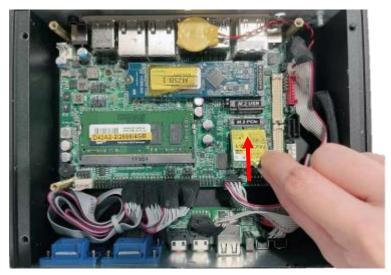
3. Insert the gold-finger side of the compatible card into the slot and press down. See to it that the golden-finger side should be fully plugged into the slot.
