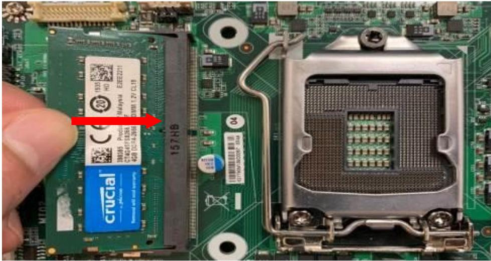
2. Insert the gold-figure side of the compatible SO-DIMM into the slot at a 30 degree angle. See to it that the break of the module fit into the notch of the slot.
