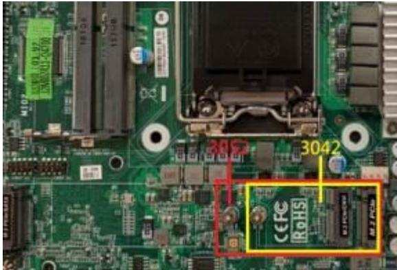
1. Locate the M.2 B-Key, type-3042/3052 slot on the board.
