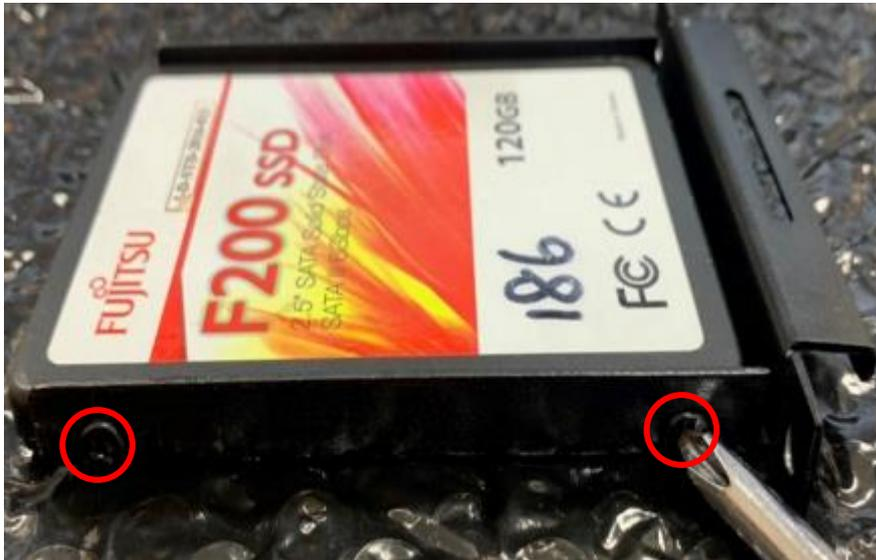
2. Lock the SATA hard disk to one of the racks by tightening the screws in the marked spots.
