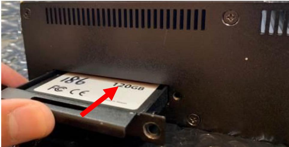
4. Insert the gold-figure side of the compatible STAT HDD into the slot.
