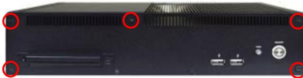
3. Remove the screws in the marked spots on the front panel.
