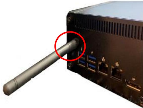
9. Connect the external Wi-Fi receiver antenna to the antenna connector on the rear panel.
