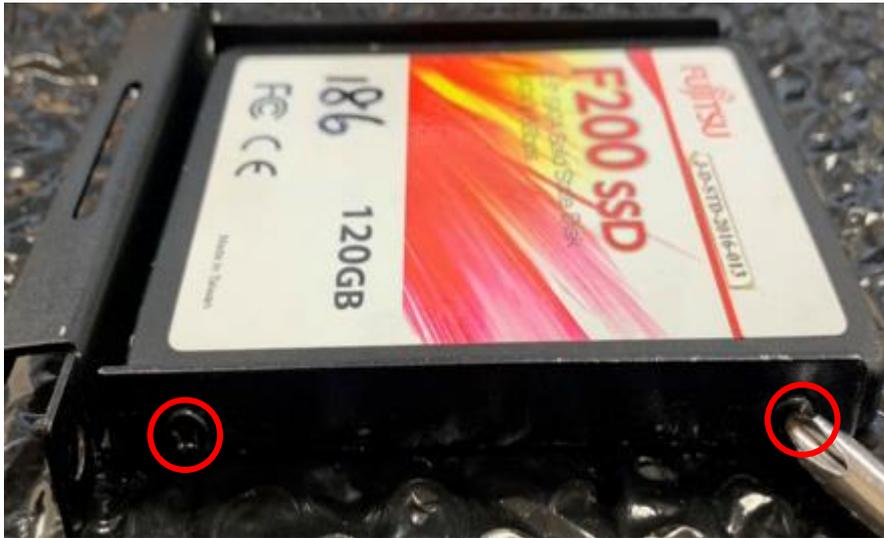
3. Lock the SATA hard disk to the other rack by tightening the screws in the marked spots.
