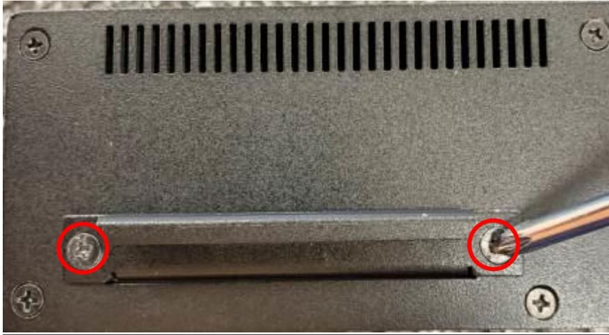
1. Remove the screws in the marked spots on the front panel.
