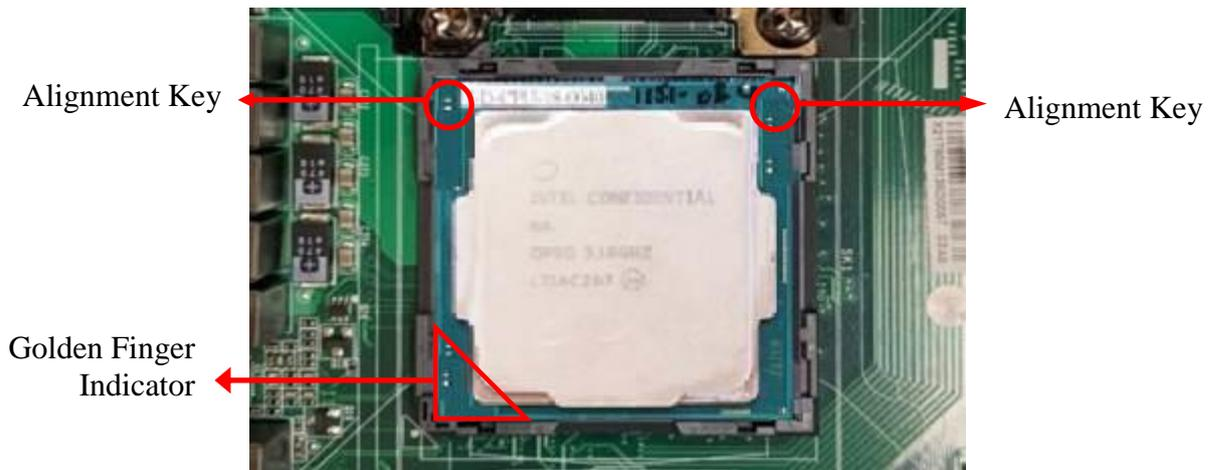
5. Make sure that Pin-1 Golden Finger Indicator in the place as shown in the above photo and match the two alignment keys on the CPU with two points of the socket. CPU can only be correctly installed in this direction. Incorrect installation might cause damage to CPU.
