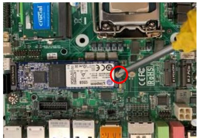
4. Install the screw back to the original spot.
