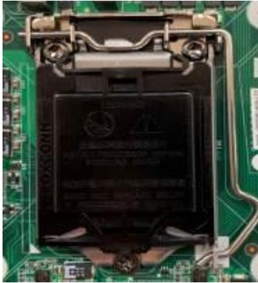
1. Find CPU socket on the board. Please make sure that CPU socket is facing towards you and the level is on your right hand side.
