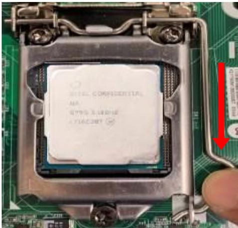
6. Put down the load plate in the direction shown above.
