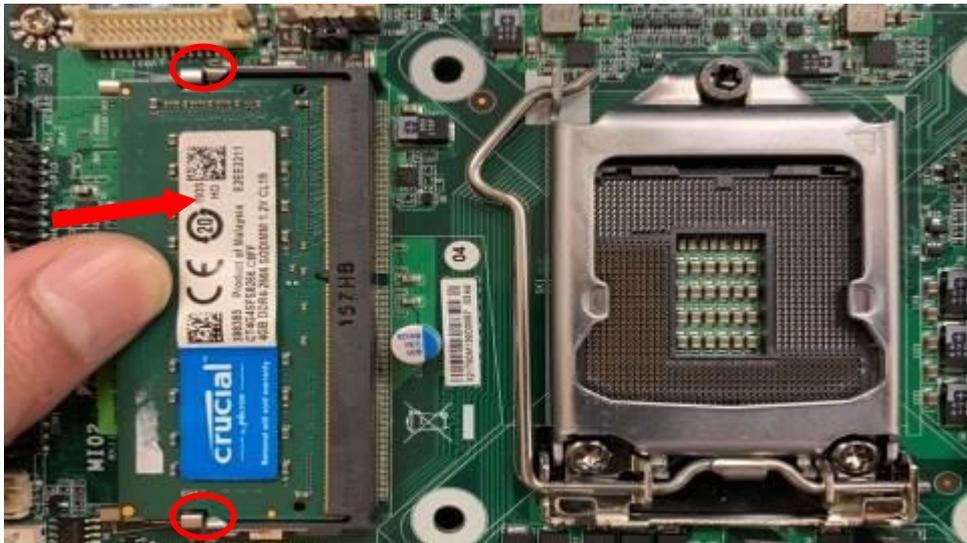
3. Press down to secure the SO-DIMM to the slot. The eject tabs will lock automatically if installing direction is correct.
