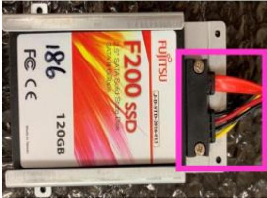
7. Plug this side of the cable to SATA power-in connector and SATA connector of the hard disk.
