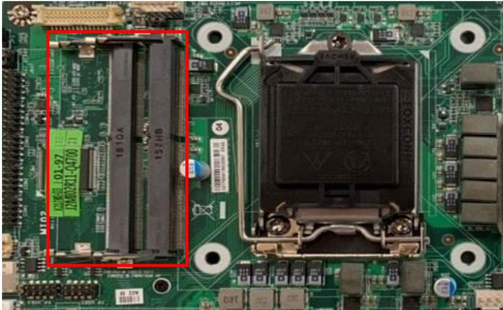
1. Find the SO-DIMM slot on the board.
