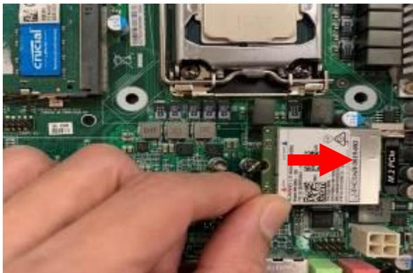
3. Insert the gold-figure side of compatible M.2 3042 card into the slot until the golden finger side fully emerged into the slot.
