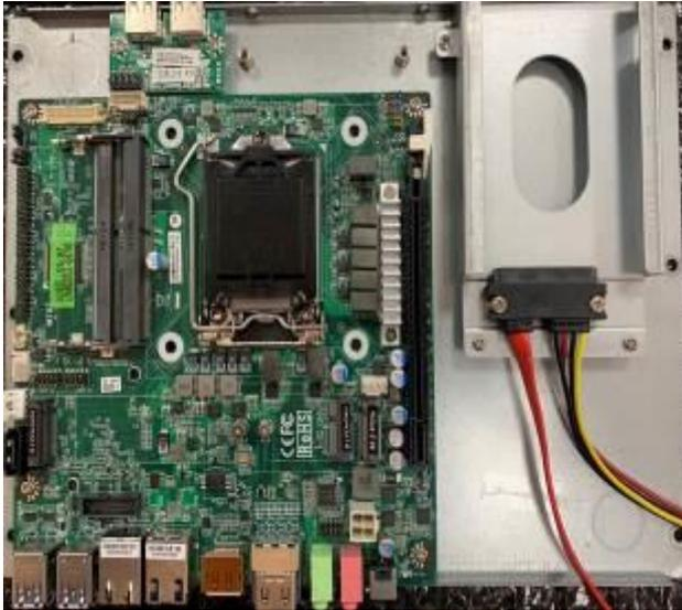
5. Remove the IO panels and lift the cover up to open the chassis. For user to have a clear view of layout, we may unplug some of the cables during installation.
