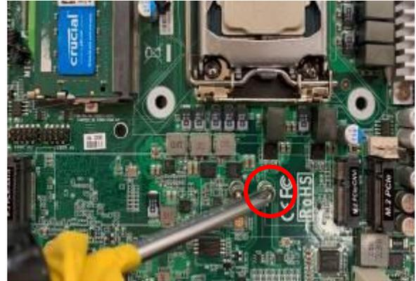
2. Remove the marked screw with a screwdriver.
