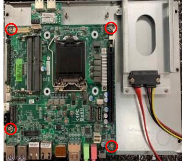
6. For CPU installation, user needs to remove the screws on the marked spots to disassemble the motherboard from chassis cover.
