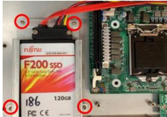
8. Lock the racks with SATA HDD installed to its original places by tightening the screws in the marked spots.
