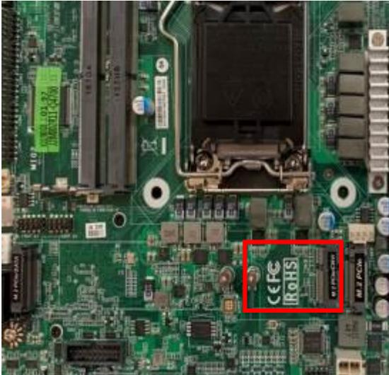
1. Locate the M.2. PCIe, type-2230 slot on the board.
