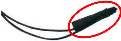
6. The metal hats on the end of the antenna string are sealed by acetate tape to avoid possible damage to the system.
