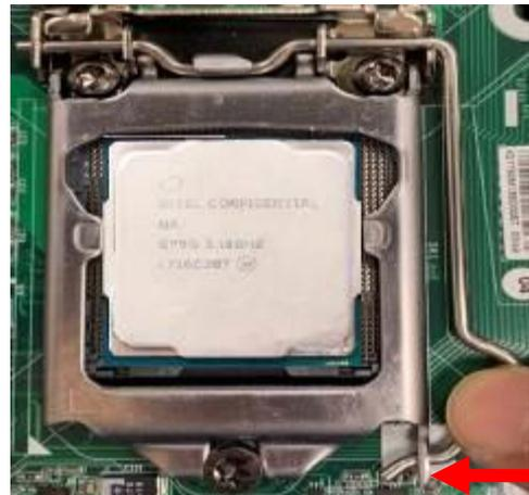
7. Press down the load level and move it leftwards to make sure it is locked under the notch.
