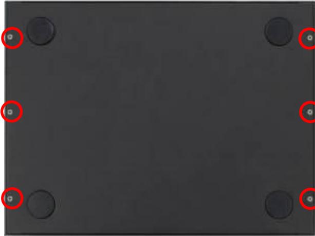
1. Locate the screws in the spots marked on the top cover of the system and unscrew them one by one.
