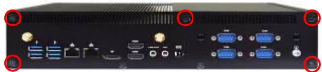
4. Remove the screws in the marked spots on the rear panel.
