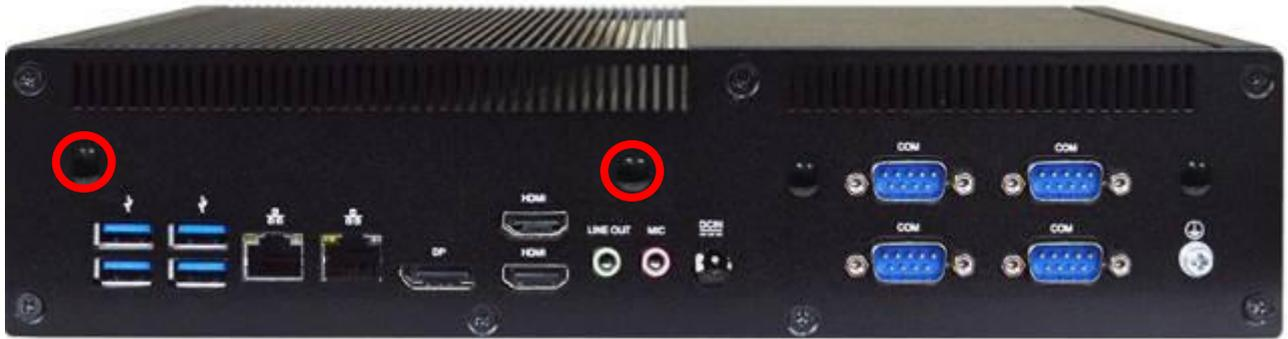
5. Locate the reserved Wi-Fi antenna holes on the back panel. Remove the dust-proof plugs on the marked spots from the panel to install the antenna, as the following details show.
