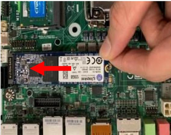
3. Insert the gold-figure side of compatible M.2 2280 card into the slot until the golden finger side fully emerged into the slot.
