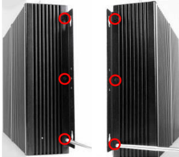
1. Install wall mount rack to the system by tightening the screws in the marked positions. Then lock the other three screws on the other side in the same way.
