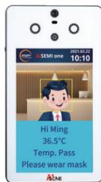
2.23 The light will turn green when the person's body temperature is within normal range, or turn red when the person's body temperature is over 37.5°C. In the case that Mask Mode is on, the light will turn green if the subject wearing a mask, or turn red if the subject not wearing any mask.
