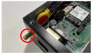
6. Push this antenna screw head into antenna hole of the rear panel from the backside of the panel.
