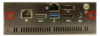
5. Locate the reserved antenna holes on the rear panel. Remove the dust-proof plugs on the marked spots from the panel to install the antenna.
