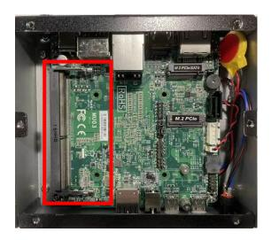
1. Locate the SO-DIMM slot on the board.
