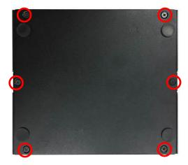
2. Locate the screws at the spots marked on the cover and unscrew them one by one.
