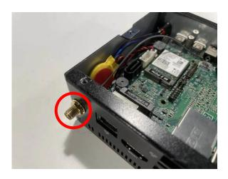
7. And then lock the antenna screw head to the front side of the rear panel with the hexagonal screw nut ② and tighten it up.
