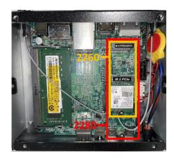
1.Locate M.2 M-Key (2260/2280) slot on the board.
