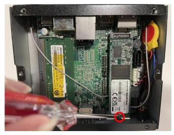
4. Lock the card to the board by tightening up the screw to the marked spot.
