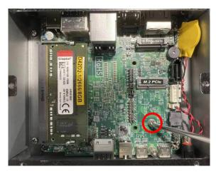
2. Remove the marked screw and use it to lock compatible card to the slot in later installation.
