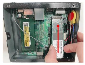
3. Insert the gold-finger side of compatible M.2 M-Key (2280) card into the slot and press down.
