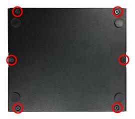
5. After completion, please tighten up the six screws on the bottom cover.
