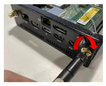
11. Connect the external Wi-Fi receiver antenna to the antenna screw head on the rear panel.
