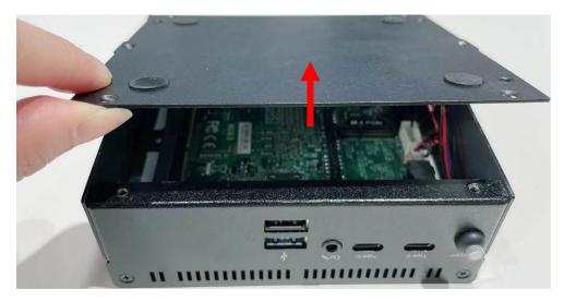
3. Lift the cover up to open the chassis.
