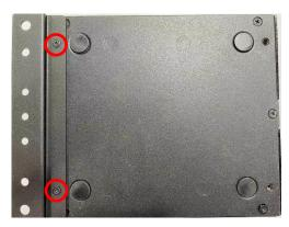
1. Install wall mount rack to the system by tightening two screws in the marked positions.
