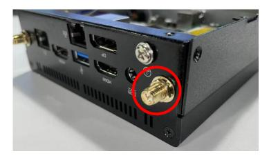
10. The rear panel with antenna screwheads installed.
