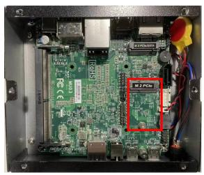
1. Locate the M.2 E-Key (2230) slot on the board. Prepare compatible M.2 E-Key (2230) card.
