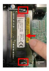
3. Press down to secure the SO-DIMM to the slot. The eject tabs will lock automatically if installing direction is correct.
