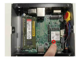
8. Press the metal hat on the end of the antenna string to corresponding antenna slot on the card as showed.
