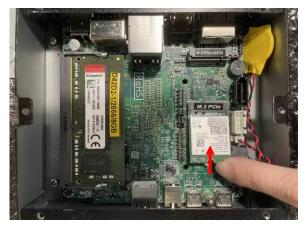
3. Insert the gold-finger side of the compatible card into the slot and press down. See to it that the golden-finger side should be fully plugged into the slot.
