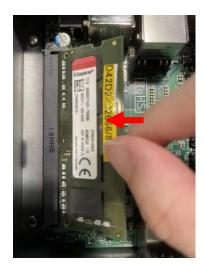
2. Insert the gold-finger side of the compatible SO-DIMM into the slot at a 30 degree.
