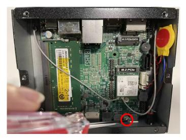
2. Remove the marked screw and use it to lock M.2 M-Key (2280) card to the slot in later installation.
