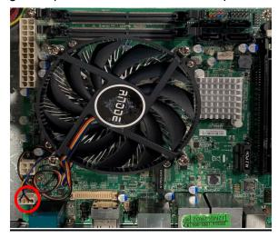
4. Connect CPU fan cable to CPU fan header of the board, as shown above.
