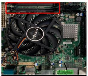
1. Find the SO-DIMM slot on the board.
