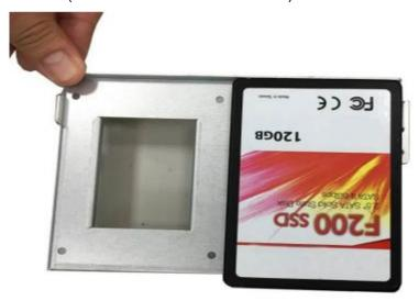
3. User can install up to  $2^*$  2.5" HDD on the tray. Adjust the 2.5" HDD on the tray until the screw holes of the tray matched those in the HDD.
