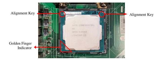
Make sure that Pin-1 Golden Finger Indicator in the place as shown in the above photo and match the two alignment keys on the CPU with two points of the socket. CPU can only be correctly installed in this direction. Incorrect installation might cause damage to CPU.
