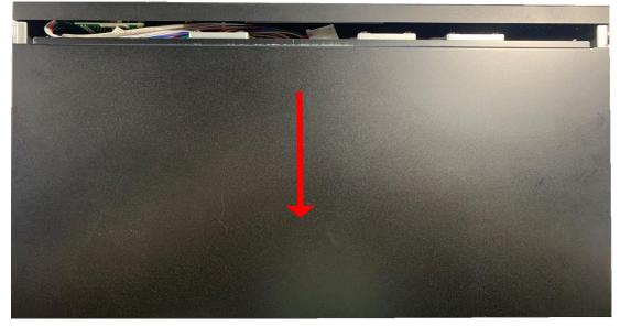
3. Push the top cover of the chassis towards the direction as the photo shows. Then lift the cover up to open the chassis.
