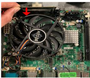
2. Insert the gold-figure side of the compatible SO-DIMM into the slot. See to it that the break of the module fit into the notch of the slot.
