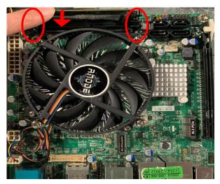
3. Press down to secure the SO-DIMM to the slot. The eject tabs will lock automatically if installing direction is correct.
