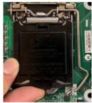
Remove the plastic protective cover from the socket (Put it to the original place if CPU is not installed. Do not touch the metal contact pins of the CPU socket).
