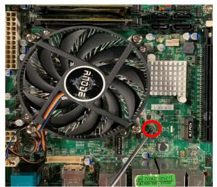
2. Remove the marked screw nut reserved for M.2 PCIe card installation first.
