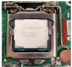
6. Put down the load plate in the direction 7. shown above.
