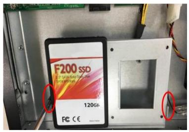
5. Put the tray with hard disk drivers installed to its original place and lock the tray to the chassis by tightening screws removed previously.
