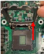
Open the level upwards about 135 degree and the metal protection plate will be pulled up at the same time.
