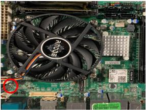
Remove the marked screw with a screwdriver.
