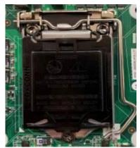
Find CPU socket on the board. Please 2. make sure that CPU socket is facing towards you and the level is on you right hand side.
