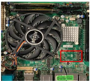
Locate the M.2. PCle, type-2230 slot on the board.
