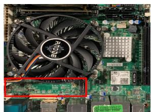
Locate the M.2 M-Key, type-2280 slot on the board.
