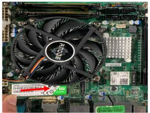
3. Insert the gold-figure side of compatible M.2 2280 card into the slot until the golden finger side fully emerged into the slot.
