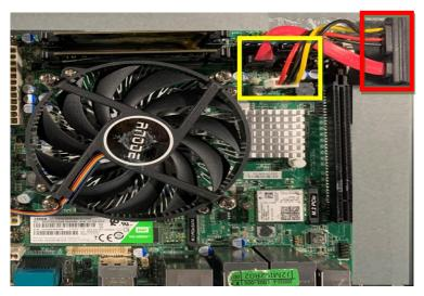
6. Connect one end of compatible SATA cable to corresponding connectors from the hard disk, and connect SATA Power cable and the other end of SATA cable to SATA port on the board as shown above.
