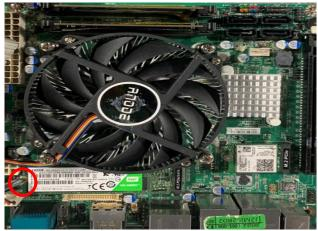
4. Install the screw back to the original spot.
