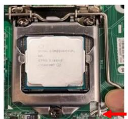
Press down the load level and move it leftwards to make sure it is locked under the notch.
