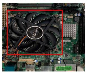
2. Put CPU fan inside the chassis and adjust it to the reserved space for fan installation.
