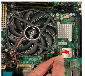
3. Insert the gold-figure side of compatible card 4. Lock the card to the board by tightening up into M.2. PCle slot. See to it that the golden-figure side is fully inserted into the slot.
