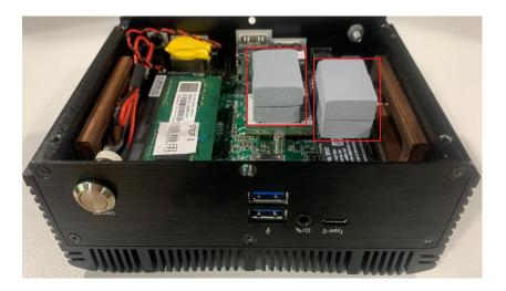
2. Stack 2 PCS of thermal conductive pads together upon M.2 M-key & M.2 B-key slots, as shown in the photo above.
