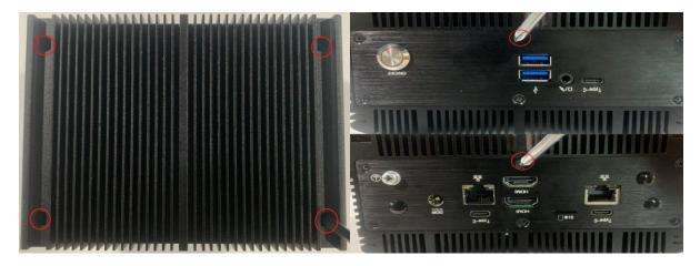
4. After completion, please tighten up the four screws on the bottom cover, one screw on the front and the other on the rear IO panels to reassemble the chassis.
