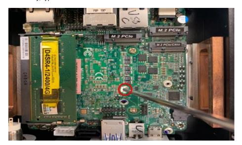
2. Remove the marked screw with a screwdriver.
