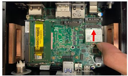
3. Insert the gold-figure side of compatible M.2 PCIe card into the slot until the golden finger side fully emerged into the slot.
