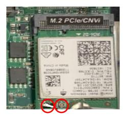
8. Press the metal hat on the end of the antenna string to corresponding antenna slot on the 2230 card as showed.
