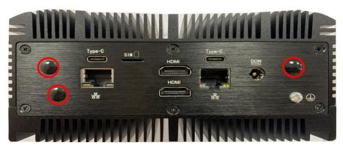
5. Locate the reserved antenna holes on the rear panel. Remove the dust-proof plugs on the marked spots from the panel to install the antenna.
