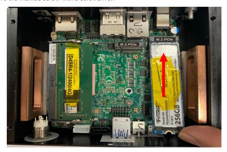
3. Insert the gold-figure side of compatible M.2 PCIe 2280 card into the slot until the golden finger side fully emerged into the slot.
