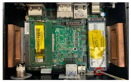
4. Install the screw back to the original spot.
