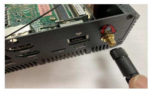
7. Connect the external Wi-Fi receiver antenna to the antenna screw head on the rear panel.
