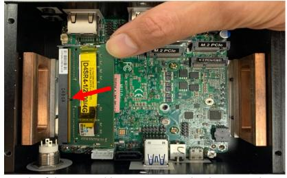
2. Insert the gold-figure side of the compatible SO-DIMM into the slot at a 30 degree angle. See to it that the break of the module fit into the notch of the slot.
