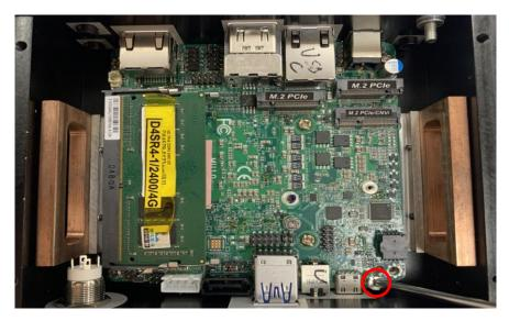
2. Remove the marked screw with a screwdriver.
