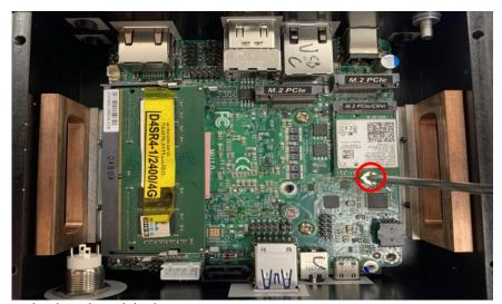
4. Install the screw back to the original spot.
