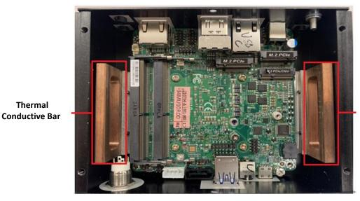
**Thermal Conductive Bar**
