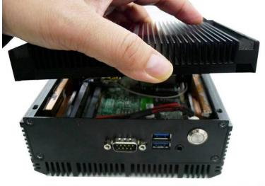
3. Lift the cover up to open the chassis.
