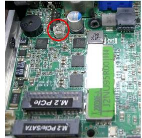
3. To install M.2 PCIe card, user need to remove the screw bolt as well.
