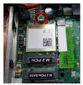
6. Install the screw bolt back to the original spot.
