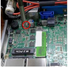
2. Remove the marked screw with a screwdriver.
