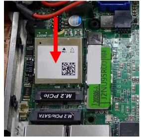
5. Insert the gold-figure side of compatible M.2 PCIe card into the slot until the golden finger side fully emerged into the slot.
