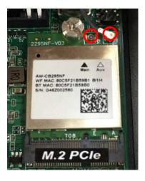
7. Press the metal hat on the end of the antenna string to corresponding antenna slot on the card as showed.
