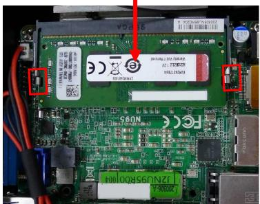
3. Press down to secure the SO-DIMM to the slot. The eject tabs will lock automatically if installing direction is correct.
