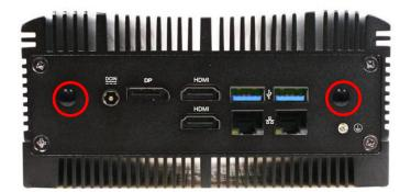
8. Locate the reserved antenna holes on the rear panel. Remove the dust-proof plugs on the marked spots from the panel to install the antenna.
