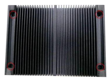
2. Locate the screws at the spots marked on this cover and unscrew them one by one to open the chassis.
