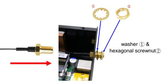
9. Push this antenna head into antenna hole of the rear panel from the backside of the panel. And then push the washer (1) through the antenna head. Lock the antenna head to the front side of the rear panel with the hexagonal screw nut(2) and tighten it up.
