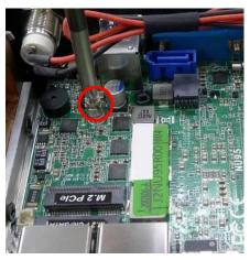
1. Locate M.2 M-key (2242) SATA slot on the 2. Remove the marked screw and use it to lock M.2 SATA board. card to the slot in later installation.
