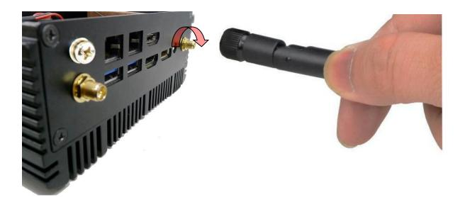
10. Connect the external Wi-Fi receiver antenna to the antenna screw head on the rear panel.
