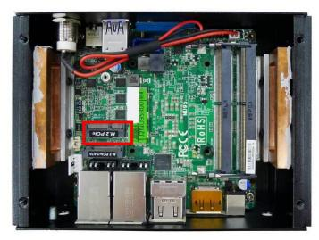
1. Locate the M.2 E-Key, type-2230 slot on the board
