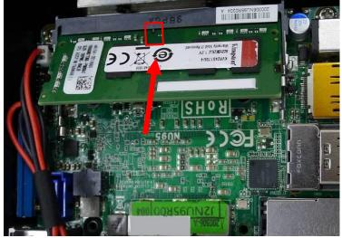
2. Insert the gold-figure side of the compatible SO-DIMM into the slot at a 30 degree angle. See to it that the break of the module fit into the notch of the slot.
