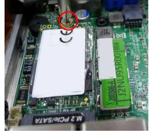
3. Insert the gold-figure side of compatible M.2 4. Lock the card to the board by tightening up the screw to SATA card into the slot until the golden finger side the marked spot. fully emerged into the slot.
