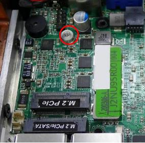
4. Use a compatible screwdriver to remover the screw bolt.
