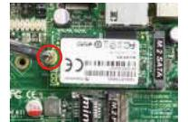
5. Align and insert the gold-figure side of the compatible M.2 SATA card into the slot. Make sure that the golden-figure side is fully inserted into the slot.
