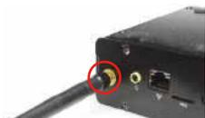
8. Connect the external Wi-Fi receiver antenna to the antenna connector on the rear panel.
