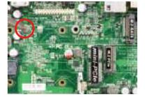
1. Locate the M.2 SATA slot on the board. Prepare compatible M.2 SATA card. Different types of cards come of different lengths. Find corresponding nut location for further installation.
