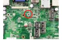
3. Remove the screw post fixed at default location (Skip step 2 & 3 and go straight to Step 4 if you are going to use the default position).
