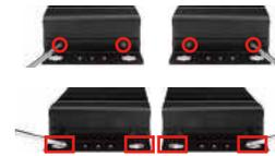
1. Install wall mount rack to the system by tightening the screws in the marked positions. Then lock the other screws on the other side in the same way.
