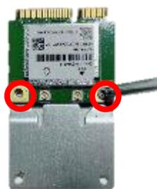
3-2. Put the card on the bracket and secure the card to the bracket by tightening up the screw to the marked spot.
