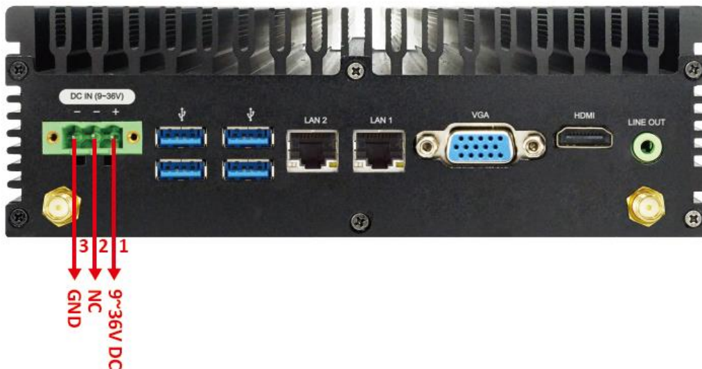
3. Rear IO diagram and DCIN power definition.
