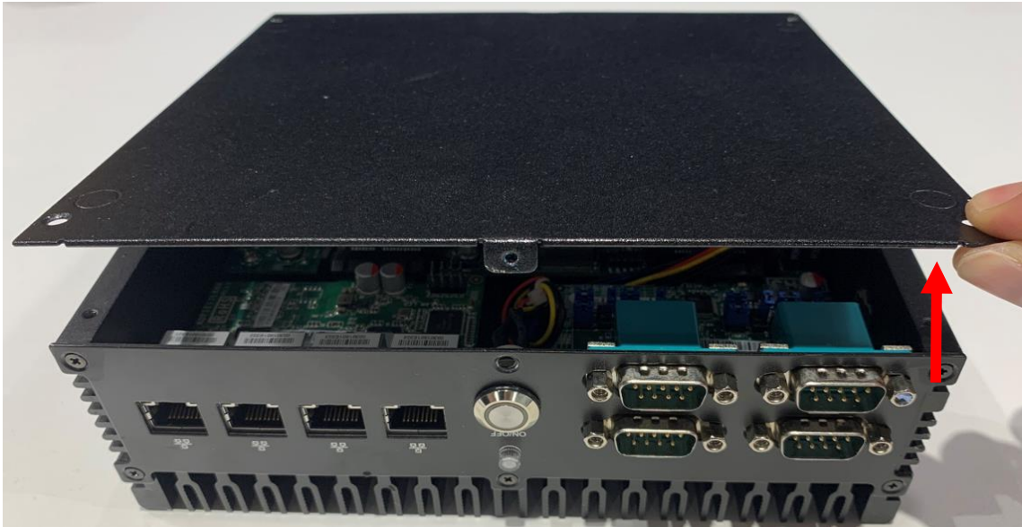
5. Lift the cover up to open the chassis.
