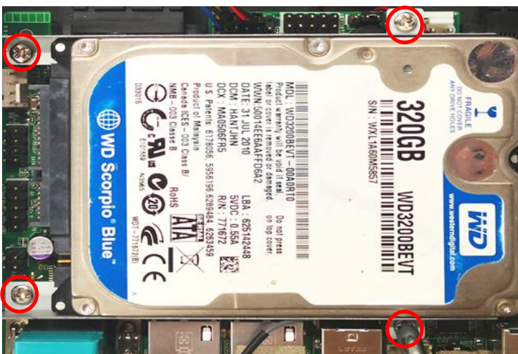
7. Lock the racks to the board by tightening up the screws in the marked spots.
