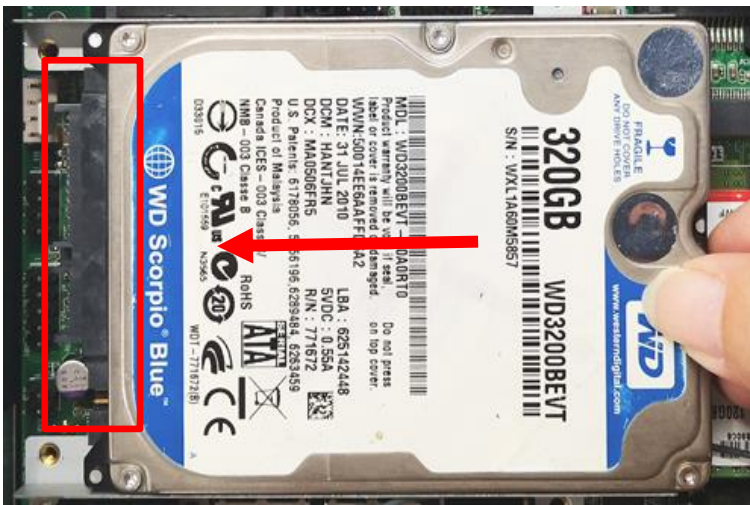
6. Push compliant HDD with rack installed to corresponding HDD connector onboard and adjust the racks to its original location before installation.
