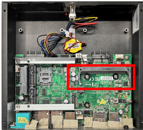
1. Locate the SO-DIMM slot on the board.
