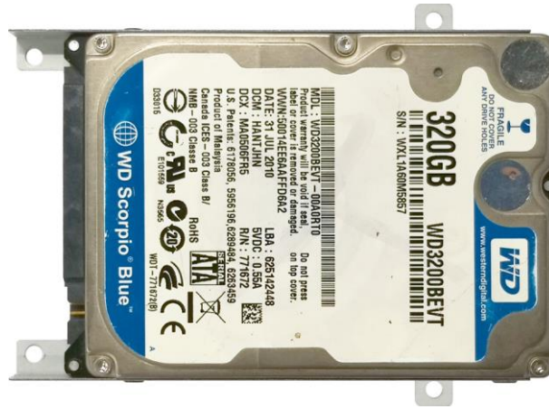
5. Hard disk drive with racks installed.
