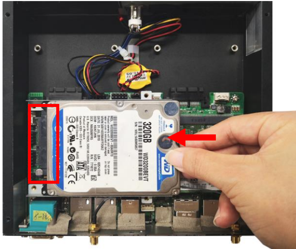
6. Push compliant HDD with rack installed to corresponding HDD connector onboard and adjust the racks to its original location before installation.
