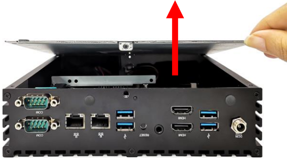
4. Lift the cover up to open the chassis.
