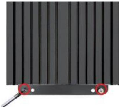
4. Tightening up the other screws on the bottom side. Check to make sure the screws are matched and fixed stably.
