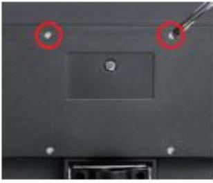
3. Unlock the reserved screws for VESA mount on the back cover of the monitor.
