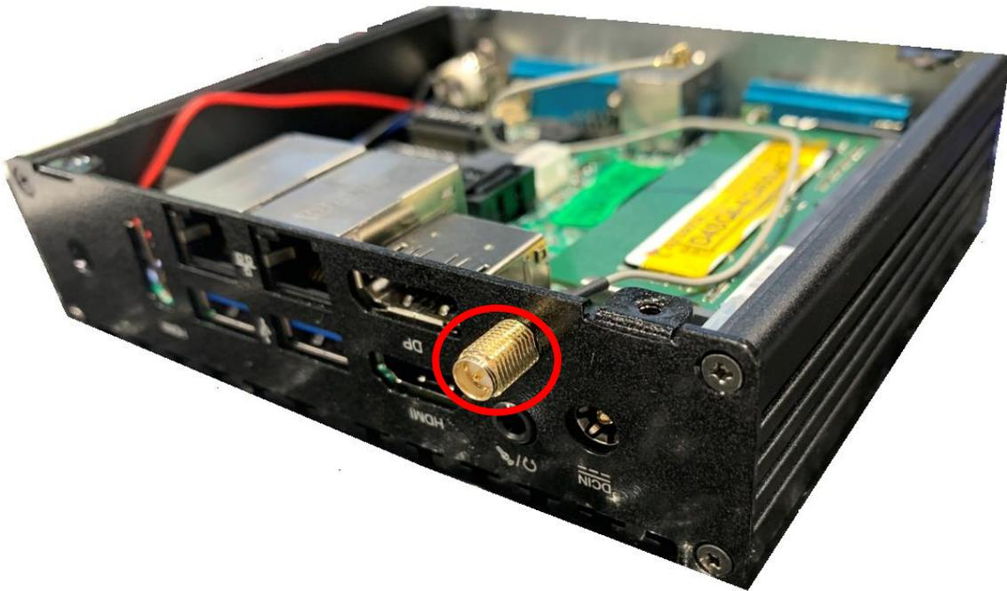
6. Push this antenna screw head into antenna hole of the rear panel from the backside of the panel.
