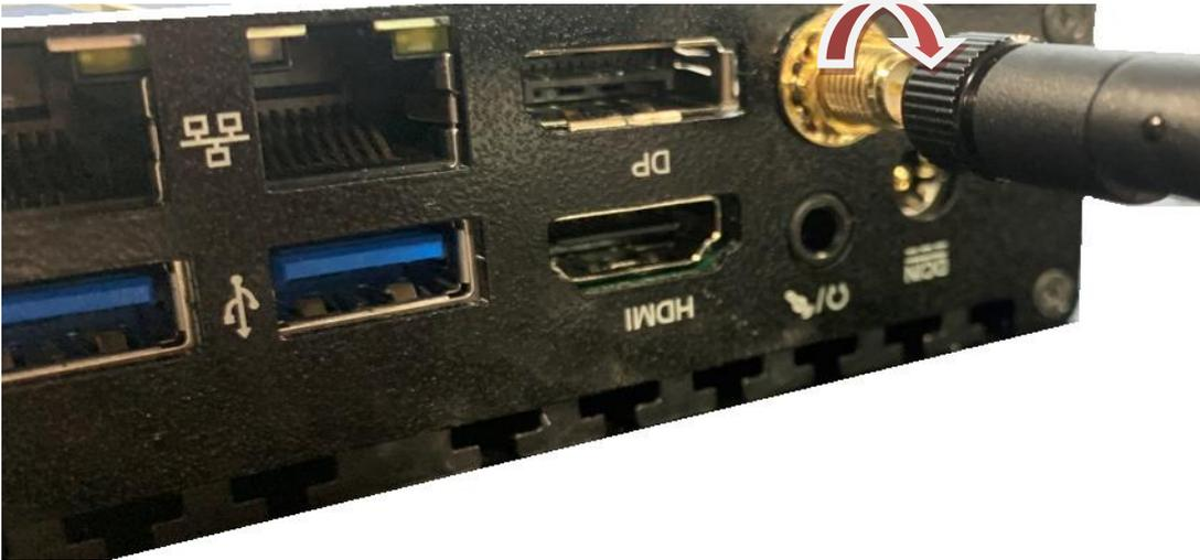
10. Connect the external Wi-Fi receiver antenna to the antenna screw head on the rear panel.
