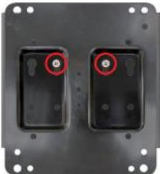
2. Place the VESA mount rack upon the cover in the direction as the photo shows. Tighten up compatible screws to lock the chassis to the rack.
