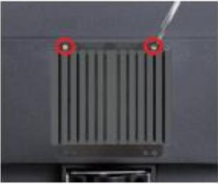
4. Adjust the chassis with VESA mount rack to the back cover of the monitor and lock it to the monitor by tightening up the above marked screws.
