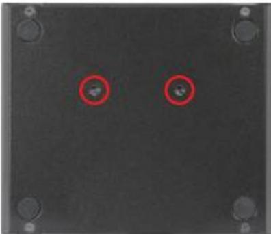
1. Locate the two screw holes reserved for VESA mount on the cover of the system. Take note of the directions of the system.
