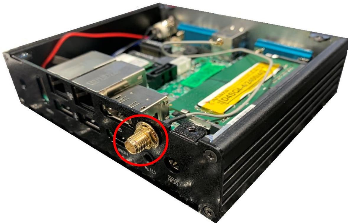
7. And then lock the antenna screw head to the front side of the rear panel with the hexagonal screw nut ② and tighten it up.
