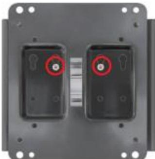
4. Install the rack to the barebone system by tightening up compatible screws in the above marked spots of the cover, as the photo shows.
