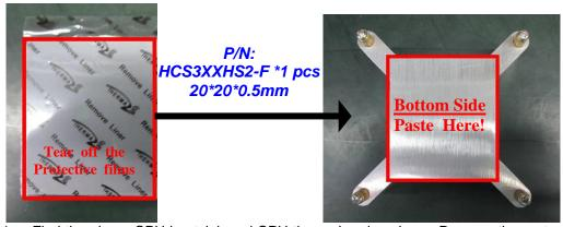
Find the above CPU heatsink and CPU thermal pad package. Remove the protective films on the both sides of the pad and apply it upon the bottom side of the heatsink for better heat conduction.
