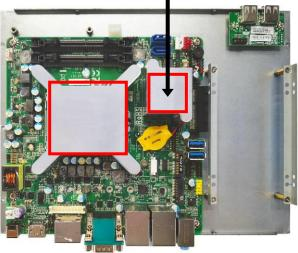
5. Apply corresponding thermal pads to chipset heat sink. When installation finished, tear off the protective film from the pads before assembling the back cover to the chassis.
