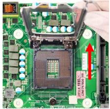
Open the level upwards about 135 degree and the metal protection plate will be pulled up at the same time.
