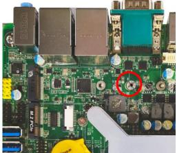
3. Remove the screw post fixed at default 4. location (Skip step 2 & 3 and go straight to Step 4 if you are going to use the default position).
