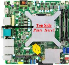
Place the CPU heatsink upon the installed CPU. The screw holes of the heatsink should match corresponding screw holes of the board. And then apply corresponding thermal pad to the top side of the heatsink as the photo shows.
