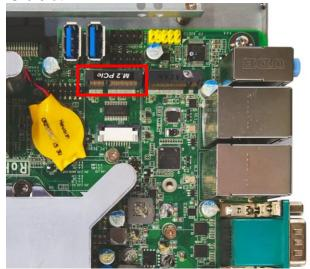
Locate the M.2. PCIe, type-2230 slot on the board.
