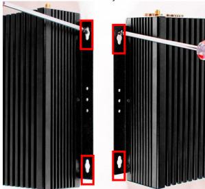
2. Wall mount the system by tightening two screws in the marked positions. Then tighten up the other two screws in the marked positions on the other rack.
