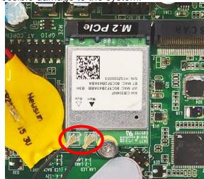
8. Press the metal hat on the end of the antenna string to the antenna slot on the card as shown.
