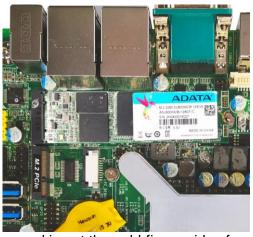
Align and insert the gold-figure side of the compatible M.2 SATA card into the slot. Make sure that the golden-figure side is fully inserted into the slot.
