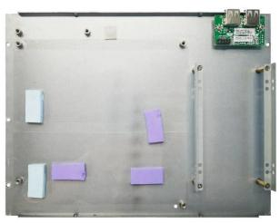
4. See to it that the silicone gel bars are in their original places for better heat dispassion and shockproof before installing the board to the system cover.
