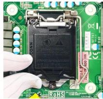
Remove the plastic protective cover from the socket (Put it to the original place if CPU is not installed. Do not touch the metal contact point of the CPU socket).
