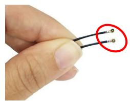
Tear off the tape to find metal hats of Wi-Fi antenna string.
