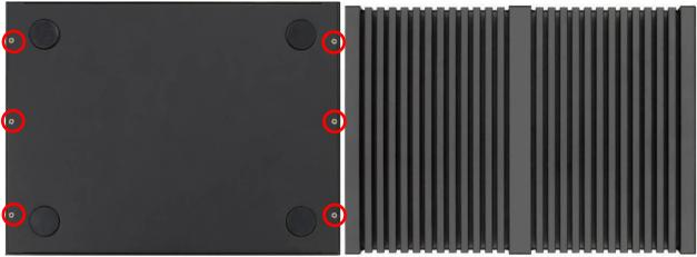
1. Locate the screws in the spots marked on the top cover of the system and unscrew them one by one.
