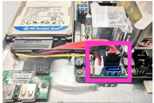
8. Plug the other sides of the cables into the SATA power connector and SATA port connector on the board.
