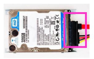
6. Plug this side of the cable to SATA 7. power-in connector and SATA connector of the hard disk.
