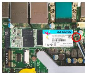
6. Lock the card to the board by tightening up the previously-removed screw nut to the marked spot.
