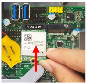
Insert the gold-figure side of compatible card into M.2. PCIe slot. See to it that the golden-figure side is fully inserted into the slot.
