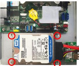
Lock the racks with SATA HDD installed to its original places by tightening the screws in the marked spots.
