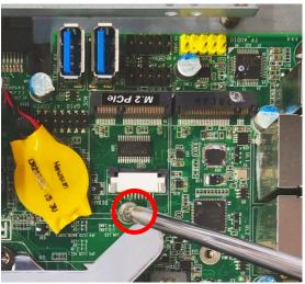
Remove the marked screw nut reserved for M.2 SATA card installation first.
