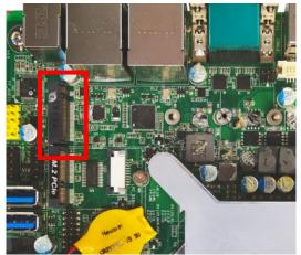
Locate the M.2 SATA slot on the board. Prepare compatible M.2 SATA or M.2 SSD card. Deferent types of cards come of different length. Find corresponding nut location for further installation.
