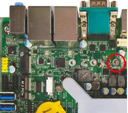
Lock the screw post into the location corresponding to the length of the module.
