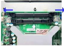
1. Find the SO-DIMM slot on the board for further installation. Open the 2\* ejects tabs before SO-DIMM installation.
