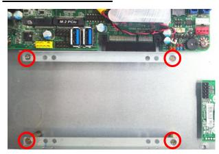
Remove the HDD racks from the cover by unscrewing the screws in the marked places.
