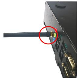
Connect the external Wi-Fi receiver antenna to the antenna connector on the rear panel.
