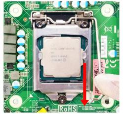
6. Put down the load plate in the direction shown 7. above.
