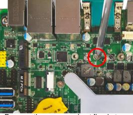
Remove the screw and nut fixed at default location (Skip step 2 & 3 and go straight to Step 4 if you are going to use the default position).
