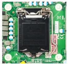
Find CPU socket on the board. Please make 2. sure that CPU socket is facing towards you and the level is on you right hand side.
