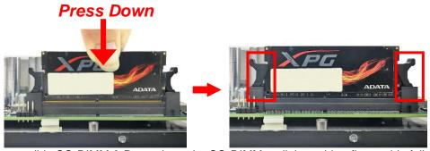
2. Adjust compatible SO-DIMM & Press down the SO-DIMM until the golden-finger side fully inserted into the slot. The eject tabs will lock automatically if installed correctly.
