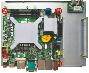
5. Remove the IO panels and lift the cover up to 6. open the chassis. For user to have a clear view of layout, we may unplug some of the cables during installation.
