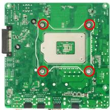
P/N: LCSC306M02-F\*4pcs (M3 Phillips round-head brass screw, Screw length 6mm, Screw tooth length 4.5mm)
