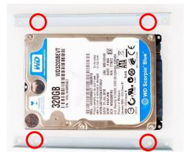
Adjust the HDD and the racks in the directions as the above photo shows.
