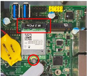
4. Lock the card to the board by tightening up the screw nut to the marked spot.
