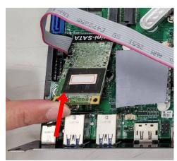
Insert the gold-figure side of the compatible Mini SATA card into the slot.
