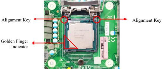
5. Make sure that Pin-1 Golden Finger Indicator in the place as shown in the above photo and match the two alignment keys on the CPU with two points of the socket. CPU can only be correctly installed in this direction. Incorrect installation might cause damage to CPU.
