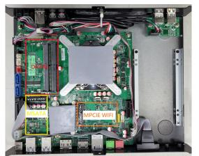
Locate the Mini SATA slot on the board.
