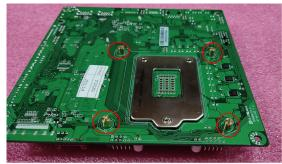
Turn over the motherboard on the platform and remover the marked screws on the back side to dissemble CPU heat sink from the board for CPU installation.
