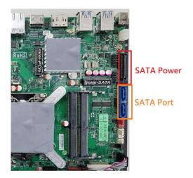
8. Plug the other side cable to the SATA power connector and SATA port connector on the board.
