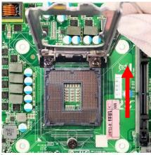
Open the level upwards about 135 degree and the metal protection plate will be pulled up at the same time.
