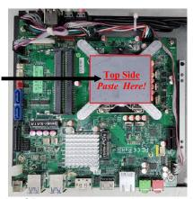
2. Place the CPU heatsink upon the installed CPU. The screw holes of the heatsink should match the heatsink as the photo shows.
