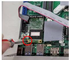
3. Lock the card to the board by tightening up the screw to the marked spot.
