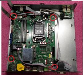
1. Unplug the connecting wires on the motherboard, and 2. then remove the 4 pcs screws and take off the motherboard.
