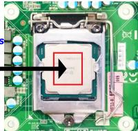
1. Find the above CPU cooler and CPU cooling pad packaging. Remove the protective film on both sides of the liner, and then apply it to the top of the CPU to achieve better heat conduction.
