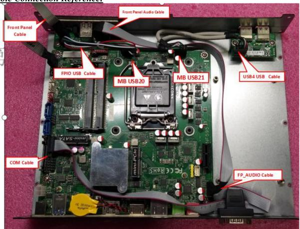
\*Note: The red wire on the cable should be connected to Pin-1.
