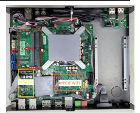
1. Find the SO-DIMM slot on the board for further installation.
