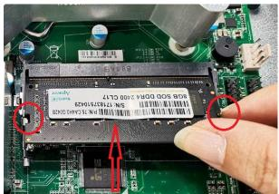
Insert the gold-figure side of the compatible SO-DIMM into the slot at a 30 degree and press down. The eject tabs will lock automatically if installed correctly.
