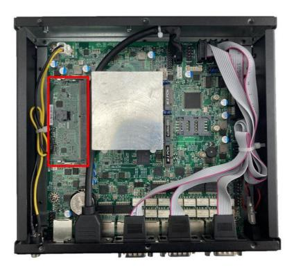
2. Insert the gold-figure side of the compatible SO-DIMM into the slot at a 30 degree angle. See to it that the break of the module fit into the notch of the slot and the golden-finger side should be fully plugged into the slot.
