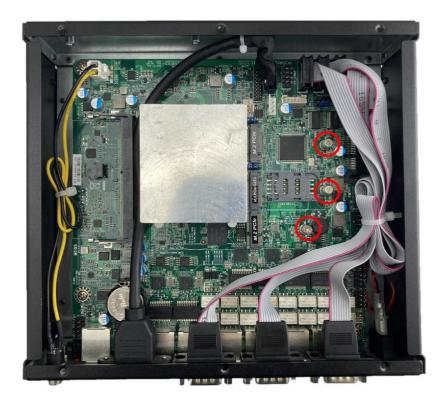
3. Insert compatible M.2 Key cards into the slots. See to it that the golden-finger side should be fully plugged into the slot.
