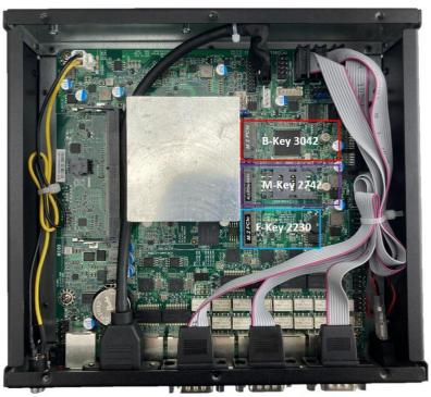
2. To install compatible cards, please remove the screws in the marked spots first.
