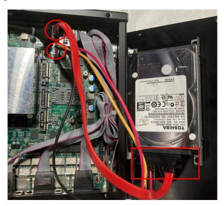
3. Make sure the SATA port of the HDD is facing the side of rear panel when closing the chassis cover as shown and tighten the 6 screws on the cover. (refer to I-1)
