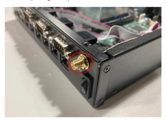
4. Press the metal hat at the end of the antenna string to corresponding antenna slot on the <u>M.2</u> <u>E-Key</u> card as shown.
