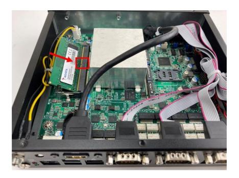
3. Press down to secure the SO-DIMM to the slot. The eject tabs will lock automatically if installing direction is correct.
