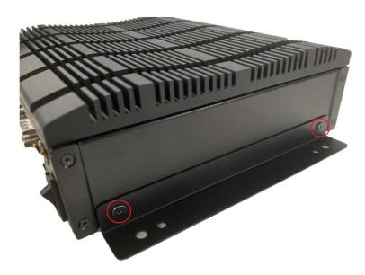
2. Wall mount the system by tightening 4 screws in the marked positions on both sides of the wall racks with the choices of large-sized and small-sized screw holes based on the project needs.
