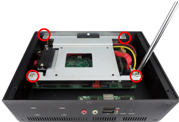
6. Remove the marked screws to disassemble the HDD tray from the system & unplug the pre-installed SATA HDD cable for further installation steps.
