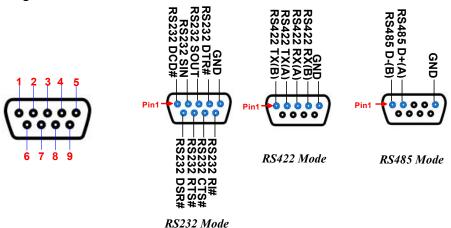
**COM1 & COM2** port can function as RS232/422/485 port. In default settings COM1/2 functions as RS232 port. With compatible COM cable COM1 can function as RS422 or RS 485 port. User also needs to go to BIOS to set '**Transmission Mode Select**' for COM1/2 at first, before using specialized cable to connect different pins of this port.
