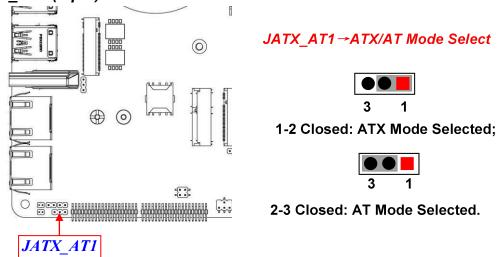
\*ATX Mode Selected: Press power button to power on after power input ready; AT Mode Selected: Directly power on as power input ready.
