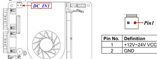
Warning: Find Pin-1 position before connecting power cable to this 3-pin power connector. WRONG INSTALLATION DIRECTION WILL DAMAGE THE BOARD!!
