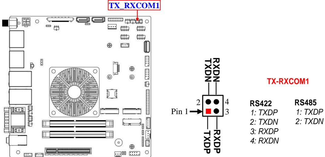
**\*Note:** COM1 RS485/RS422 function is extended on TX\_RXCOM1 header and realized by JCOM1 jumper selection and BIOS settings; after JCOM1 selection made, user needs to go to BIOS to set 'Transmission Mode Select' as [RS422] or [RS485] for COM1 as well (refer to Page-36).
