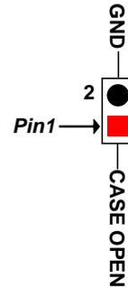
**Pin (1-2) Short:** When Case open function pin short to GND, the Case open function was detected. When used, needs to enter BIOS and enable '**Case Open Detect**' function. In this case if your case is removed, next time when you restart your computer, a message will be displayed on screen to inform you of this.
