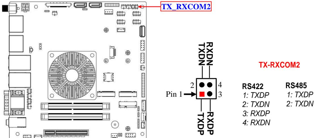
**\*Note:** COM2 RS485/RS422 function is extended on TX\_RXCOM2 header and realized by JCOM2 jumper selection and BIOS settings; after JCOM2 selection made, user needs to go to BIOS to set 'Transmission Mode Select' as [RS422] or [RS485] for COM2 as well (refer to Page-37).
