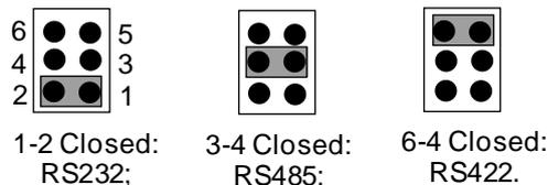
**\*Note:** COM1 RS485/RS422 function is extended on TX\_RXCOM1 header and realized by JCOM1 jumper selection and BIOS settings; after JCOM1 selection made, user also needs to enter BIOS settings 'Advanced Menu' → 'Serial Port 1 Configuration' → 'Transmission Mode Select' and set it as [RS232], [RS232] or [RS485] mode.
