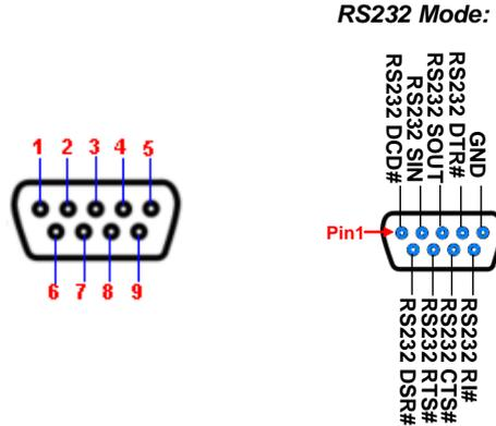
**\*Note:** **COM1** RS485/RS422 function is extended on **TX\_RXCOM1** header and realized by **JCOM1** jumper selection and **BIOS settings**; after **JCOM1** selection made, user also needs to enter BIOS settings 'Advanced Menu' → 'Serial Port 1 Configuration' → 'Transmission Mode Select' and set it as **[RS232]**, **[RS232]** or **[RS485]** mode.
