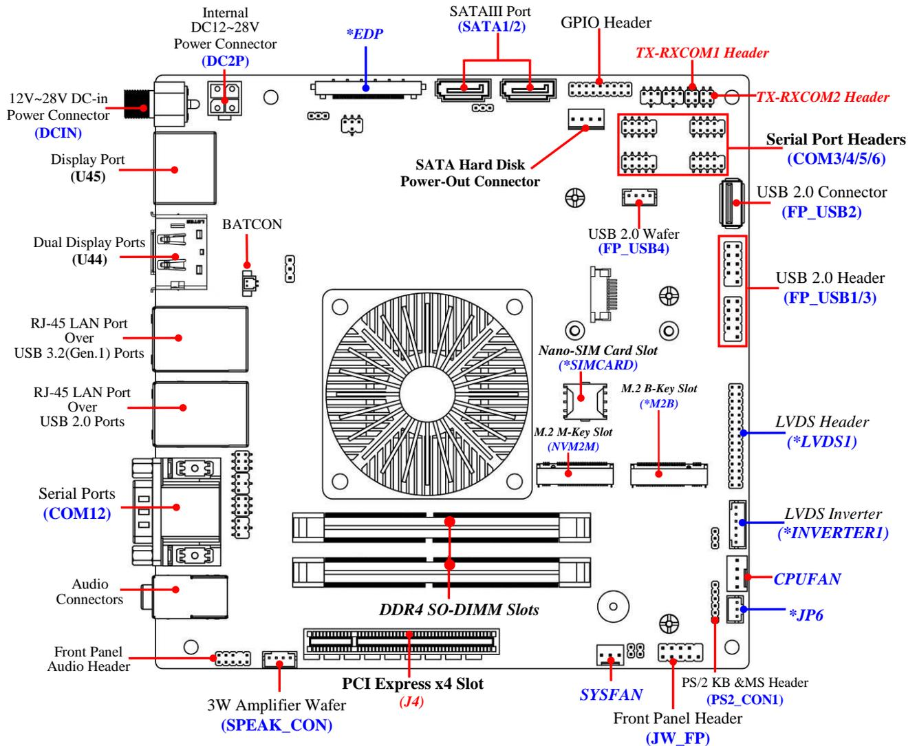
**\*Note:** SIMCARD slot only work when compatible Nano-SIM card installed & 4G/5G LAN card installed in M2B slot.
