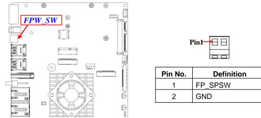
*Warning:* Power connection to Rear *DCIN1* and Internal *FPW\_SW* can not be made simultaneously. Apply compatible power cable to only one of them to power on the system.
