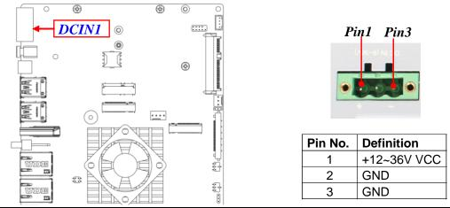
Warning: Find Pin-1 position before connecting power cable to this 3-pin power connector. WRONG INSTALLATION DIRECTION WILL DAMAGE THE BOARD!!
