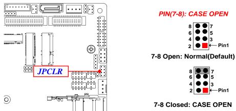
**Pin (7-8) Closed**: When Case open function pin short to GND, the Case open function was detected. When used, needs to enter BIOS and enable 'Case Open Detect' function. In this case if your case is removed, next time when you restart your computer, a message will be displayed on screen to inform you of this.
