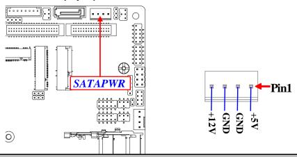
**Warning:** Make sure that Pin-1 of compatible SATA Power out connector is inserted into corresponding Pin-1 of **SATAPWR** connector to avoid possible damage to the board and hard disk driver!
