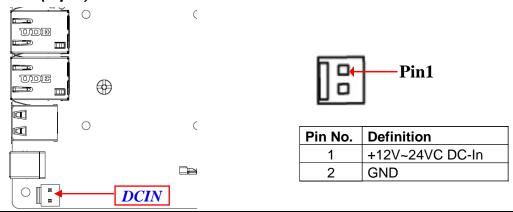
Warning: Find Pin-1 position before connecting power cable to this 2-pin power connector. WRONG INSTALLATION DIRECTION WILL DAMAGE THE BOARD!!
