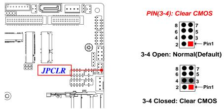
\*Note: Due to Intel MRC Code design factor, the first reboot after Clear CMOS will run a full **Memory Sizing**, and the boot time will take about **40** seconds (normal reboot time length, not function failure).
