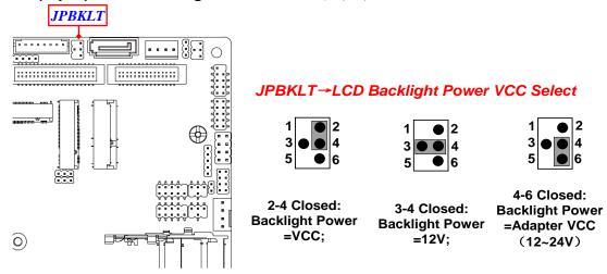
\*Note: In the case that JPBKLT is set as Pin(4-6) closed, backlight power VCC is the same as adapter voltage value (wide voltage range from 12V to 24V).
