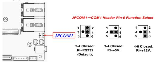
\*Note:Maximum current limit is 500mA while using 5V or 12V.
