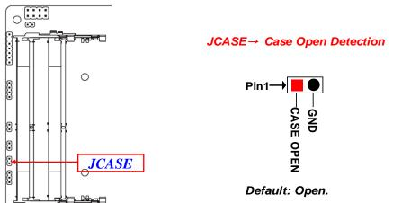
Pin 1-2 Short: When Case open function pin short to GND, the Case open function was detected. When Used, needs to enter BIOS and enable 'Case Open Detect' function. In this case if your case is removed, next time when you restart your computer, a message will be displayed on screen to inform you of this.
