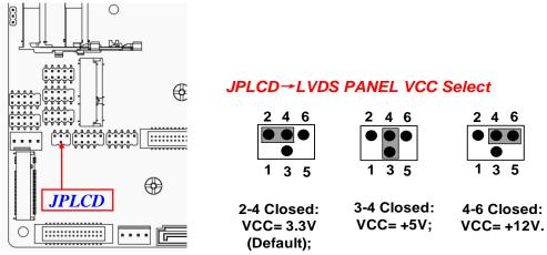
\*Note: Maximum current limit is 2A while using 3.3V, 5V or 12V.
