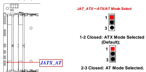
\*ATX Mode Selected: Press power button to power on after power input ready;
