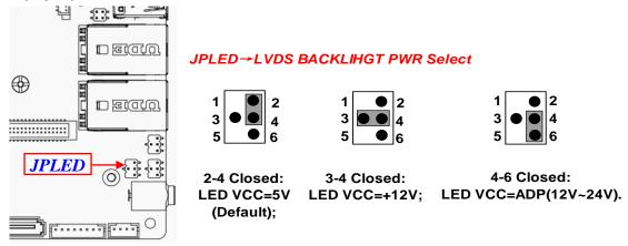
\*Note: Maximum current limit is 2A while using 5V or 12V.
