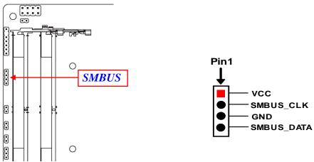
\*Note: Maximum current limit is 300mA while using 5V working voltage.
