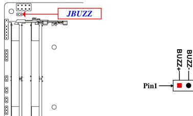
\*Note: Maximum current limit is 60mA while using 5V working voltage.
