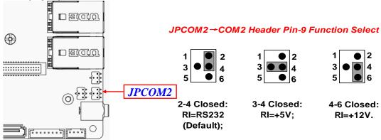
\*Note:Maximum current limit is 500mA while using 5V or 12V.
