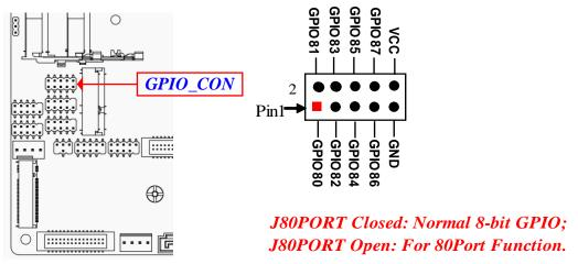
\*Note:1.Maximum current limit is 1A while using 5V working voltage; 2.Please refer to Page-11 J80PORT jumper settings for GPIO\_CON 80Port or GPIO Port function select.
