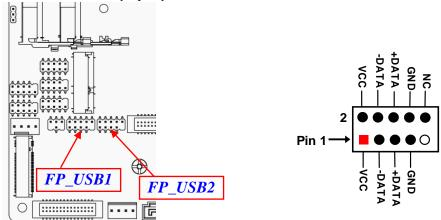
\*Note: Maximum current limit is 1.5A in total while using 5V working voltage.
