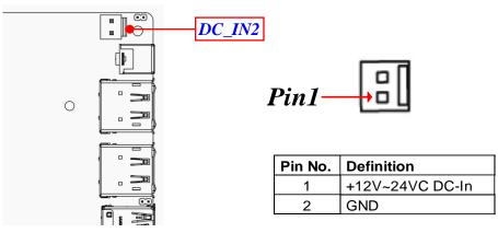
Warning: Find Pin-1 position before connecting power cable to this 2-pin power connector. WRONG INSTALLATION DIRECTION WILL DAMAGE THE BOARD!!
