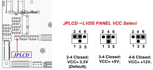
\*Note: Maximum current limit is 2A while using 3.3V, 5V or 12V.
