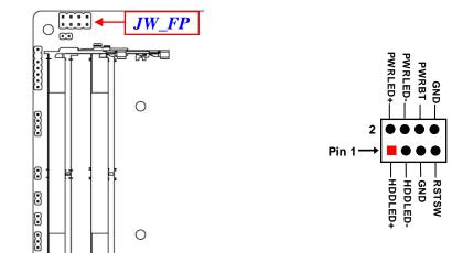
\*Note: Maximum current limit is **1A** while using 5V working voltage.
