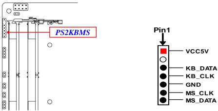
\*Note: Maximum current limit is 500mA while using 5V working voltage.
