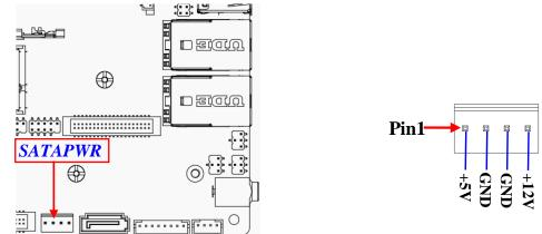
**Warning:** Make sure that Pin-1 of compatible SATA Power out connector is inserted into corresponding Pin-1 of **SATAPWR** connector to avoid possible damage to the board and hard disk driver!
