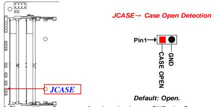
**Pin 1-2 Short:** When Case open function pin short to GND, the Case open function was detected. When Used, needs to enter BIOS and enable 'Case Open Detect' function. In this case if your case is removed, next time when you restart your computer, a message will be displayed on screen to inform you of this.
