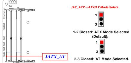
\*ATX Mode Selected: Press power button to power on after power input ready; AT Mode Selected: Directly power on as power input ready.
