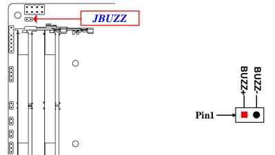
\*Note: Maximum current limit is 60mA while using 5V working voltage.
