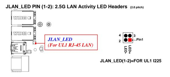
\*Note: Maximum current limit is 300uA while using 3.3V working voltage.
