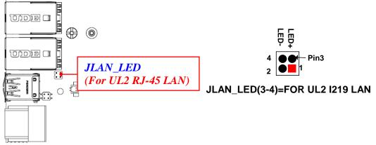
\*Note: Maximum current limit is 300uA while using 3.3V working voltage.
