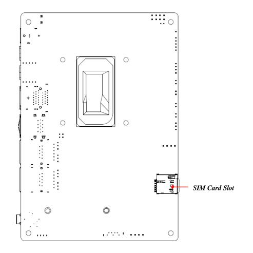
\*Note: SIM card slot (along with M.2 B-key)
