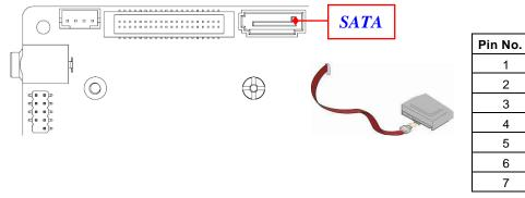
(4) SATAPWR (4-pin): SATA HDD Power-Out Connector
