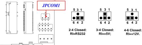
\*Note:Maximum current limit is 500mA while using 5V or 12V.
