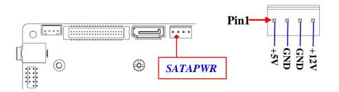
**Warning:** Make sure that Pin-1 of compatible SATA Power out connector is inserted into corresponding Pin-1 of **SATAPWR** connector to avoid possible damage to the board and hard disk driver!
