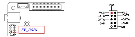
\*Note: Maximum current limit is 1.5A in total while using 5V working voltage.
