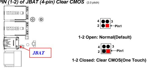
PIN (1-2) of JBAT (4-pin) Clear CMOS (2.0 pitch)
