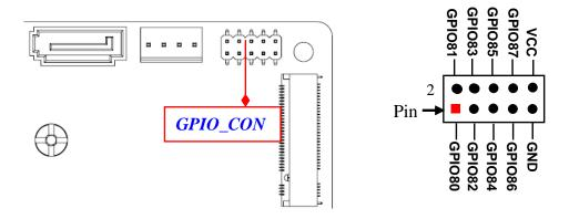
J80PORT Closed: Normal 8-bit GPIO; J80PORT Open: For 80Port Function.
