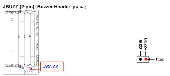
\*Note: Maximum current limit is 60mA while using 5V working voltage.
