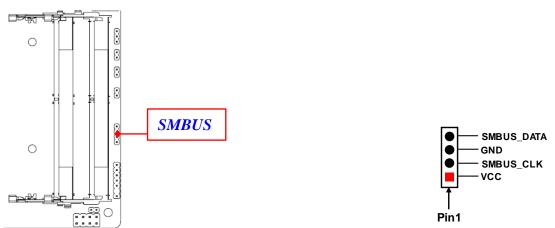
\*Note: Maximum current limit is **300mA** while using 5V working voltage.
