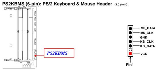
\*Note: Maximum current limit is **500mA** while using 5V working voltage.
