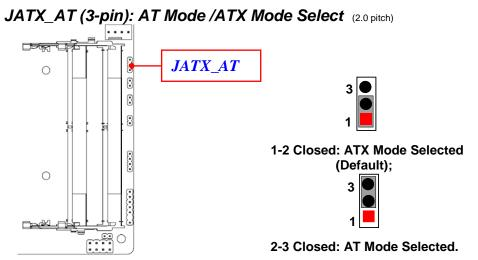
\*ATX Mode Selected: Press power button to power on after power input ready; AT Mode Selected: Directly power on as power input ready.
