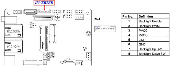
*Warning!* Find *Pin-1* location of the inverter and make sure that the installation direction is correct! Otherwise serious harm will occur to the board/display panel!!
