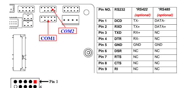
\*Note: COM1 header can function as RS232/422/485 port header. In normal settings COM1 functions as RS232 header. With compatible COM cable COM1 can function as RS422 or RS 485 header. User also needs to go to BIOS to set 'Transmission Mode Select' for COM1 at first, before using specialized cable to connect different pins of this port.
