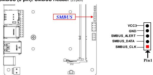
SMBUS (5-pin): SMBUS Header (2.0 pitch)
