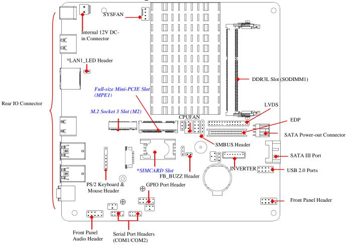
Note: SIMCARD slot only work when compatible SIM card installed & 3G LAN card installed in full-size Mini-PCIE (MPE1) slot.
