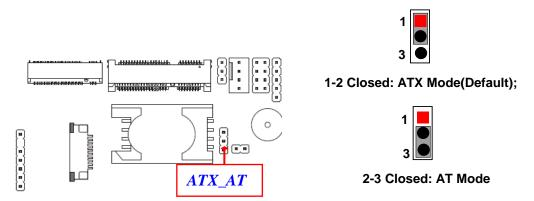
\*ATX Mode Selected: Press power button to power on after power input ready; AT Mode Selected: Directly power on as power input ready.
