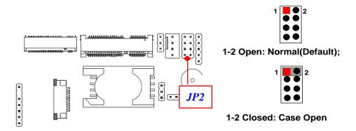
**Pin (1-2) Close:** When Case Open function pin short to GND, the Case Open function was detected. When Used, needs to enter BIOS and enable 'Case Open Detect' function. In this case if your case is removed, next time when you restart your computer, a message will be displayed on screen to inform you of this.
