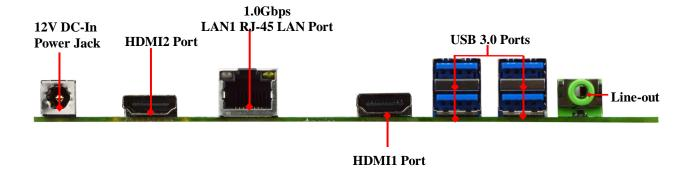
**Warning!!**The board has a 12V DC-in power connector (**DCIN3**) in I/O back panel and an internal 12V power connector (DCIN2). User can only connect one type of compatible power supply to one of them to power the system.
