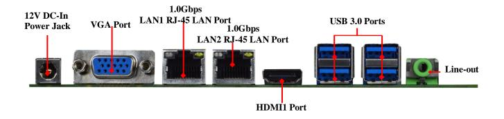
**Warning!!**The board has a 12V DC-in power connector (**DCIN3**) in I/O back panel and an internal 12V power connector (DCIN2). User can only connect one type of compatible power supply to one of them to power the system.
