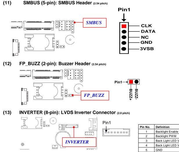
Warning! Find Pin-1 location of the inverter and make sure that the installation direction is correct!Otherwise serious harm will occur to the board/display panel!!
