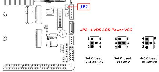
\*Note: Maximum current limit is 2A while using 3.3V/5V/12V working voltage \*Warning! Wrong voltage setting will result in screen burn out.
