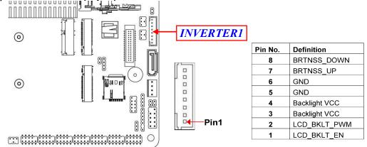
**Warning!** Find **Pin-1** location of the inverter and make sure that the installation direction is correct! Otherwise serious harm will occur to the board/display panel!!
