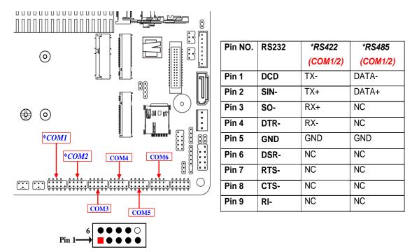
\*Notice: COM1/2 header can function as RS232/422/485 port header. In normal settings COM1/2 functions as RS232 header. With compatible COM cable COM1/2 can function as RS422 or RS 485 header. User also needs to go to BIOS to set 'Transmission Mode Select' for COM1 or COM2 at first, before using specialized cable to connect different pins of this port.
