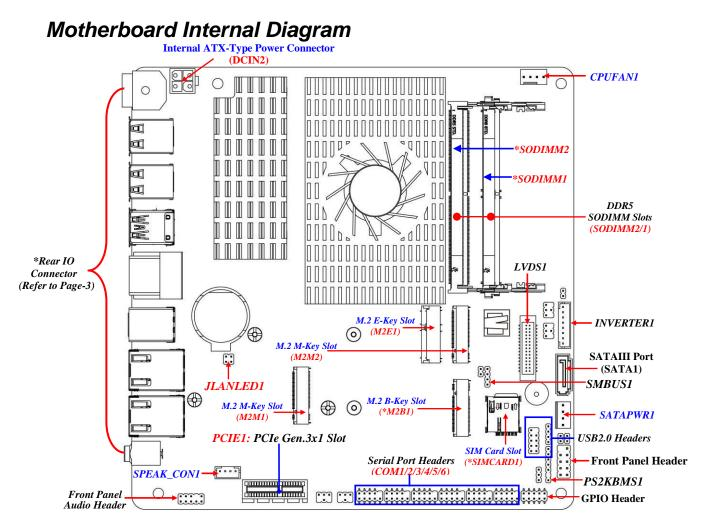
\*Note: 1.SIMCARDB1 slot only work when compatible SIM card installed & 4G/5G LAN card installed in M2B1 M.2 B-key slot.
