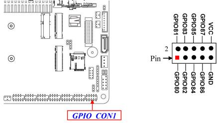
\*Note: GPIO\_CON1 can function as Debug 80 port or GPIO port via J80PORT1 jumper setting (refer to Page-10 for J80PORT1 description).
