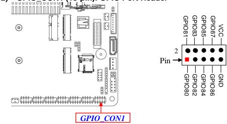
\*Note: GPIO CON1 can function as Debug 80 port or GPIO port via J80PORT1 jumper setting (refer to Page-10 for J80PORT1 description).
