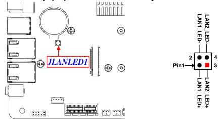
\*Note: Maximum current limit is 300uA while using 3.3V working voltage.
