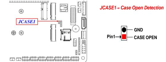
**Pin (1&2) Short**: When Case open function pin short to GND, the Case open function was detected. When used, needs to enter BIOS and enable 'Case Open Detect' function. In this case if your case is removed, next time when you restart your computer, a message will be displayed on screen to inform you of this.
