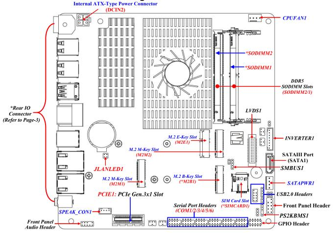
\*Note: 1.SIMCARDB1 slot only work when compatible SIM card installed & 4G/5G LAN card installed in M2B1 M.2 B-key slot.
