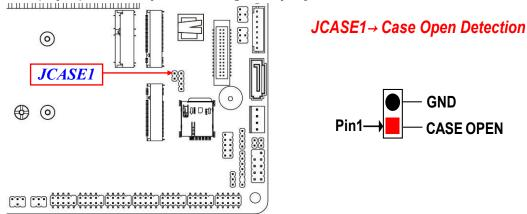
**Pin (1&2) Short**: When Case open function pin short to GND, the Case open function was detected. When used, needs to enter BIOS and enable 'Case Open Detect' function. In this case if your case is removed, next time when you restart your computer, a message will be displayed on screen to inform you of this.
