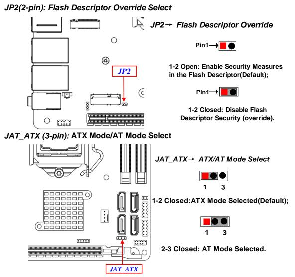
\*ATX Mode Selected: Press power button to power on after power input ready;
