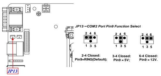
\*Note:Maximum current limit is 500mA while using 5V or 12V.
