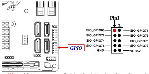
\*Note: Maximum current limit is **1A** while using 5V working voltage.
