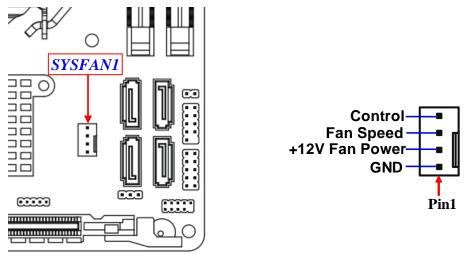
\*Note: Maximum current limit is **1.5A** while using 12V working voltage.
