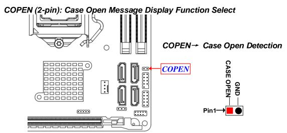
**Pin (1&2) Closed**: When Case open function pin short to GND, the Case open function was detected. When used, needs to enter BIOS and enable 'Case Open Detect' function. In this case if your case is removed, next time when you restart your computer, a message will be displayed on screen to inform you of this.
