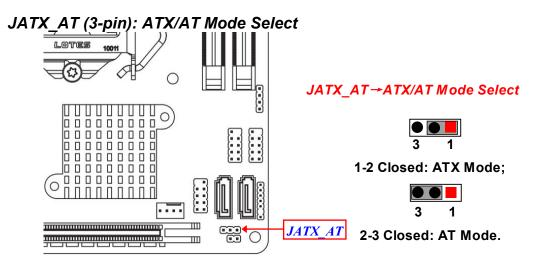
\*ATX Mode Selected: Press power button to power on after power input ready; AT Mode Selected: Directly power on as power input ready.
