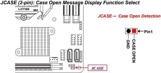
**Pin (1&2) short**: When Case open function pin short to GND, the Case open function was detected. When used, needs to enter BIOS and enable 'Case Open Detect' function. In this case if your case is removed, next time when you restart your computer, a message will be displayed on screen to inform you of this.
