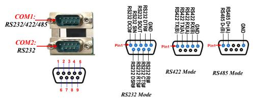
COM1 port can function as RS232/422/485 port. In normal settings COM1 functions as RS232 port. With compatible COM cable COM1 can function as RS422 or RS 485 port. User also needs to go to BIOS to set 'Transmission Mode Select' for COM1 at first, before using specialized cable to connect different pins of this port.
