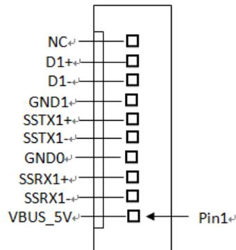
**\*Note:** Maximum current limit is 1.5A while using 5V working voltage
