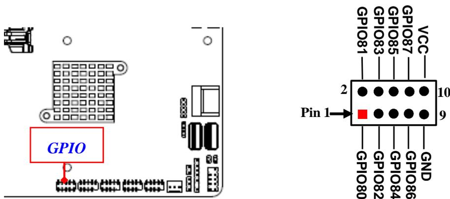
*\*Note: Maximum current limit is 1.5A while using 5V working voltage.*
