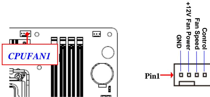
*\*Note: Maximum current limit is 0.5A while using 5V working voltage*
