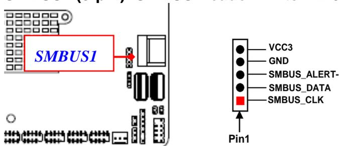
*\*Note:* Maximum current limit is 0.3A while using 5V working voltage
