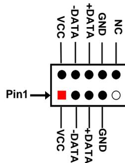
**\*Note:** Maximum current limit is 1.5A while using 5V working voltage. MM10-H6100/6102 only has FP\_USB4/5.
