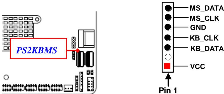
*\*Note:* Maximum current limit is 500mA while using 5V working voltage
