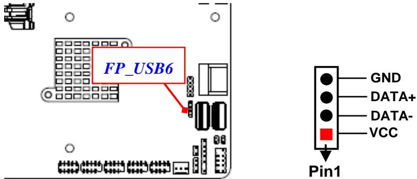
*\*Note: Maximum current limit is 1.5A while using 5V working voltage*
