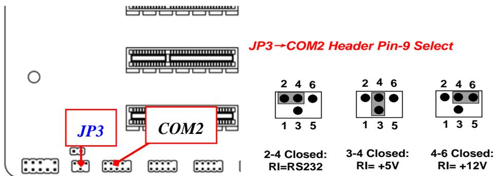
**\*Note:** Maximum current limit is 500mA while using 5V or 12V.
