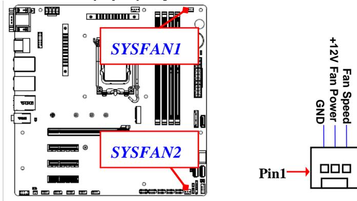
*\*Note: Maximum current limit is 0.5A while using 5V working voltage*
