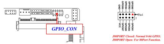
\*Note: Please refer to **Pege-11 J80PORT** jumper setting for GPIO\_CON header **GPIO Port** or **80 Port** function select.
