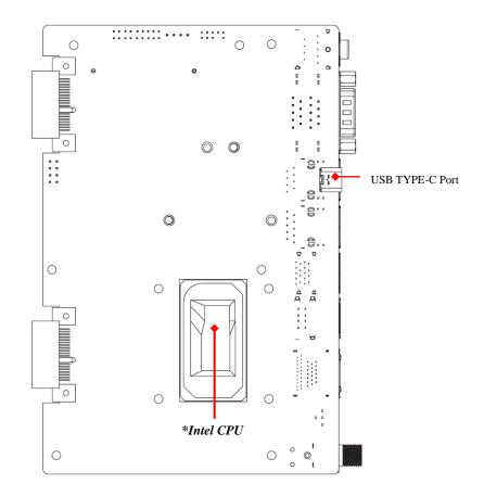
\*Note: CPU is the most important part of the board and very fragile to any possible harm. Make sure that there is no damage to the CPU during any installation procedures!
