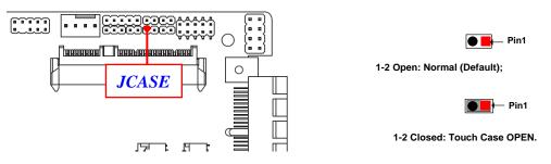
**Pin 1-2 Short**: When Case open function pin short to GND, the Case open function was detected. When Used, needs to enter BIOS and enable 'Case Open Detect' function. In this case if your case is removed, next time when you restart your computer, a message will be displayed on screen to inform you of this.
