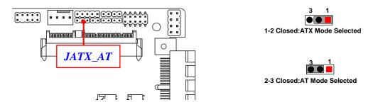
**ATX Mode Selected**: Press power button to power on after power input ready; **AT Mode Selected**: Directly power on as power input ready.
