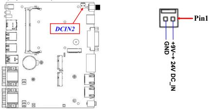
**Warning:** Power connection to Rear **DCIN1** and Internal **DCIN2** can not be made simultaneously. Apply compatible power cable to only one of them to power on the system.
