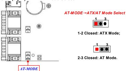
\*ATX Mode Selected: Press power button to power on after power input ready;
