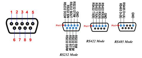
COM1 port can function as RS232/422/485 port. In normal settings COM1 functions as RS232 port. With compatible COM cable they can function as RS422 or RS 485 port. User also needs to go to BIOS to set '**Transmission Mode Select**' at first, before using specialized cable to connect different pins of this port.
