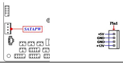
**Warning:** Make sure that Pin-1 of compatible SATA Power connector is inserted into corresponding Pin-1 of SATAPW to avoid possible damage to the board and hard disk driver!
