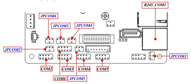
JPCOM2→COM2 Pin-9 VCC JPCOM3→COM3 Pin-9 VCC JPCOM4→COM4 Pin-9 VCC JPCOM5→COM5 Pin-9 VCC JPCOM6→COM6 Pin-9 VCC
