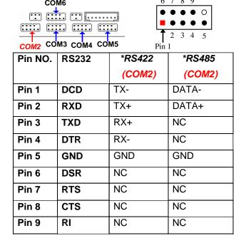
\*Notice: COM2 header can function as RS232/422/485 port. In normal settings COM1 functions as RS232 port. With compatible COM cable COM2 can function as RS422 or RS 485 port. User also needs to go to BIOS to set 'Transmission Mode Select' for COM2 as [RS422] or [RS485] for boards that support RS422/485 function before connecting compatible COM cable to COM2 header.
