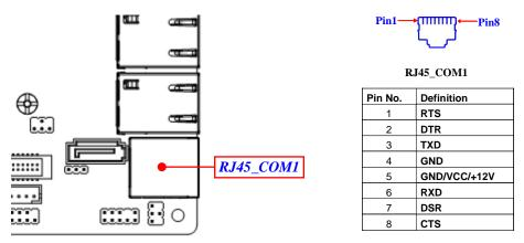
**Note:** Please set **Pin (2-4)** of Jumper **JPCOM1** as closed, when apply Console cable to RJ45-COM1 port (refer to page-12).
