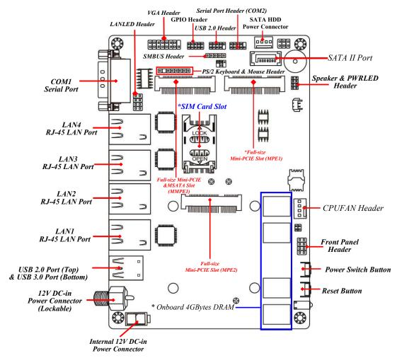
Note: SIM card slot only work when compatible SIM card installed & 3G LAN card installed in MPE1 Mini-PCIE slot.
