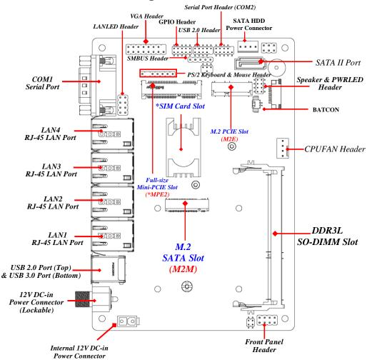
\*Note: SIM card slot only work when compatible SIM card installed & 3G LAN card installed in MPE2 full-size Mini-PCIE slot.
