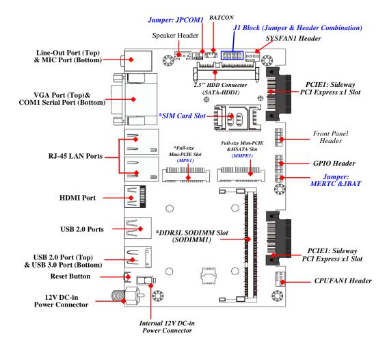
Note: 1. The memory module should be DDR3L 1.35V SODIMM and not exceeding 8GB total capacity. 2. SIM card slot only work when compatible SIM card installed & 3G LAN card installed in MPE1 Mini-PCIE slot.
