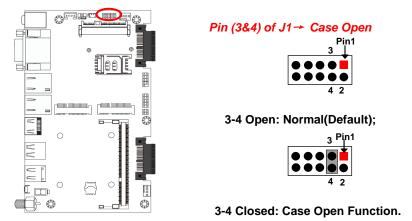
**Pin (3&4) Closed**: When Case open function pin short to GND, the Case open function was detected. When Used, needs to enter BIOS and enable 'Case Open Detect' function. In this case if your case is removed, next time when you restart your computer, a message will be displayed on screen to inform you of this.
