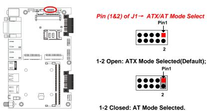
\*ATX Mode Selected: Press power button to power on after power input ready; AT Mode Selected: Directly power on as power input ready. Pin (3&4)of J1 (10-pin): Case Open Message Display Function Select (2.54 pitch)
