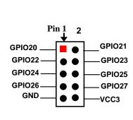
(3) Pin(5&6) & Pin(7&8) of J1 (10-pin): LAN Activity LED Headers (2.54 pitch)
